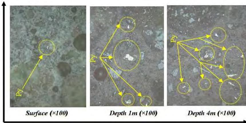
**Figure 3** Mineralogical images of tailings samples (Py: Pyrite), at different depths of the old tailings disposal site.
