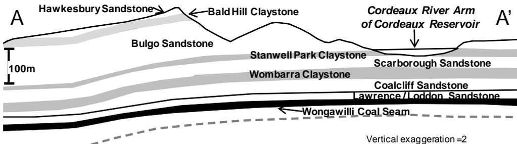
Figure 3 Cross section through Area 2 and Cordeaux River Arm of Cordeaux Reservoir (see location of cross section on Figure 1B).
