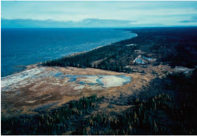
Figure 9 Upward discharge of saline water and accumulation of mineral precipitate at an open artesian (flowing) borehole at the south shore of Great Slave Lake, NWT, Canada (picture: K.U. Weyer, 1977; Weyer 2010a)
