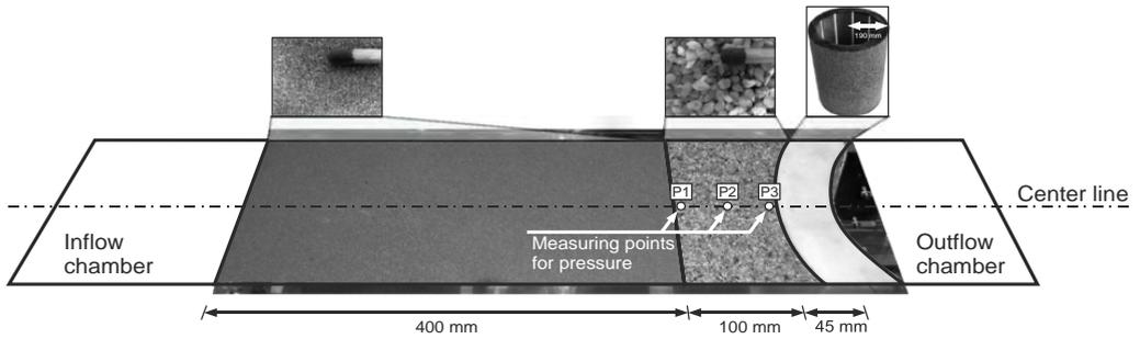
**Figure 2** Perspective top view of the material assembled in the flow channel. The flow direction is from left to right. The width and height of the channel are 200 mm each. The pressure measurement points P1-P3 actually lie on the bottom of the channel and are projected to the top for illustration purposes only.
