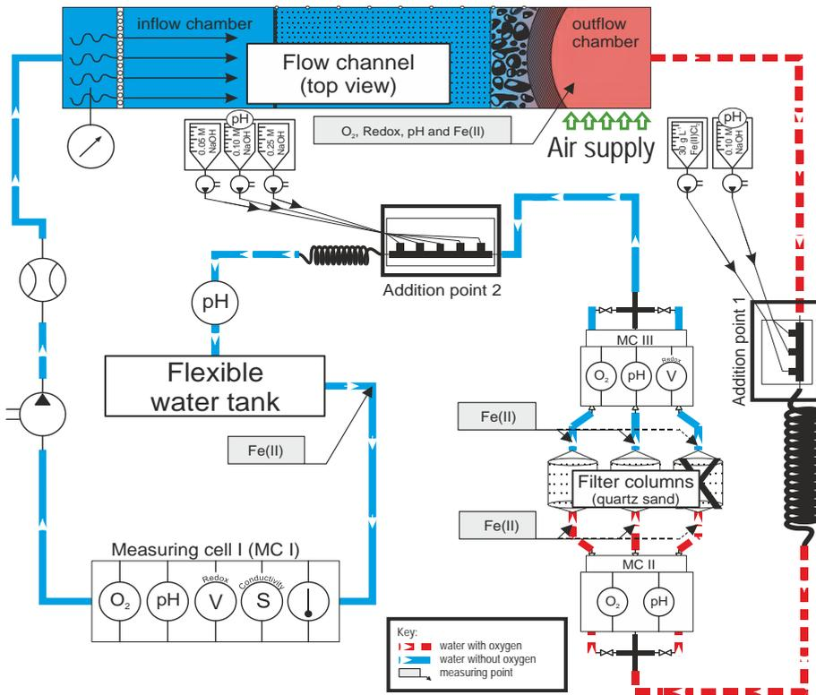
**Figure 1** Experimental setup with illustration of the flow direction and the zones of O<sub>2</sub>-bearing and O<sub>2</sub>-free water. During the test period each of the filter columns can be exchanged by a third one. A 150 L flexible water tank is used as a storage reservoir for volume fluctuations and for buffering the effects of addition point 2.
