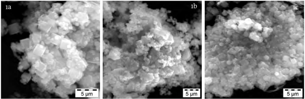
**Figure 4** SEM images of zeolite A synthesized using different solvents 1a) pure water, 1b) CNW and 1c) AMD with sonication at 100 °C for one hour using raw unfiltered fly ash slurry.
