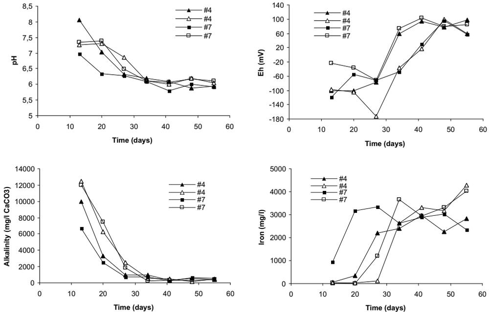
**Figure 2** Evolution of pH, Eh, alkalinity and iron concentration in treated effluent using mixtures #4 and #7.
