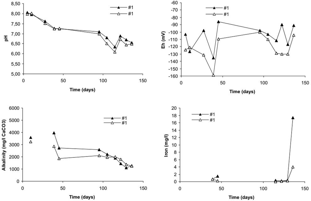
Figure 3 Evolution of pH, Eh, alkalinity and total iron concentration in treated effluent using mixture #1.
