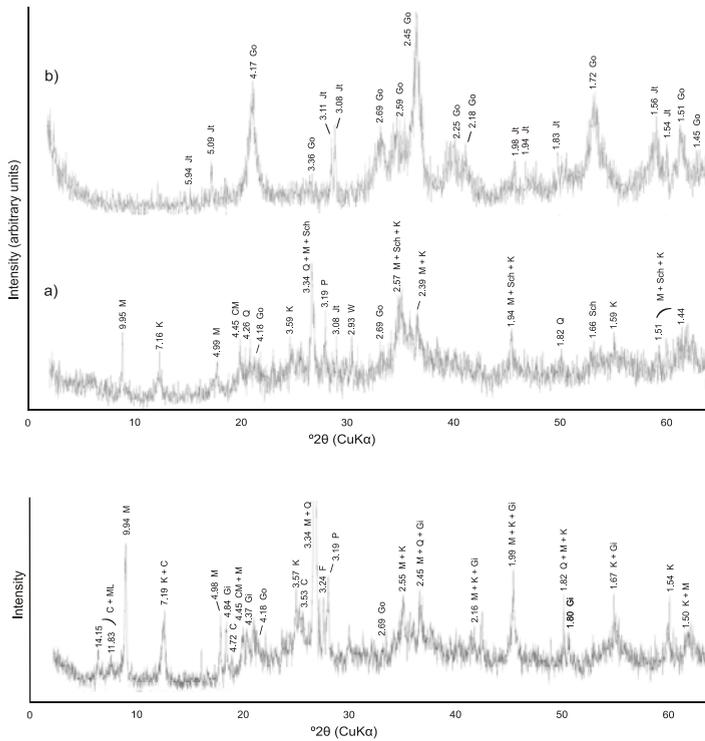
**Figure 2** XRD pattern of samples collected in the Poço Negro creek, showing *d* values in Å. a) V3 sample; b) V5 sample. K = Kaolinite; see other symbols in tab.1.
