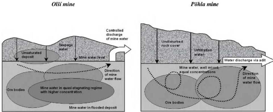
Figure 2 Schematic of water flow in the flooded mines of Olší and Pöhla
