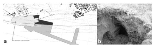
Figure 3 Dominion No.3 Site - mining hazards: a) hazard map; b) hidden shallow workings
