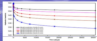
Hydraulic head vs. Elapsed time intervals for various rates of pumping
