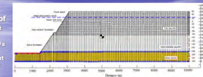
246 nodes,120 rect. Elements;60m thick & 10000m long aquifer
