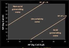
When a given tailings fall in the uncertainty interval, or when there is a need for a better understanding of the future geochemical behavior, kinetic tests are recommended.
