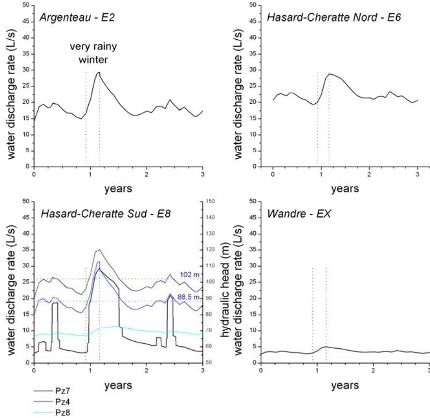
Figure 9. Very rainy winter scenario - Simulated water discharge rates
