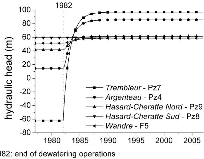
Figure 6. Groundwater rebound scenario - Simulated hydraulic heads
