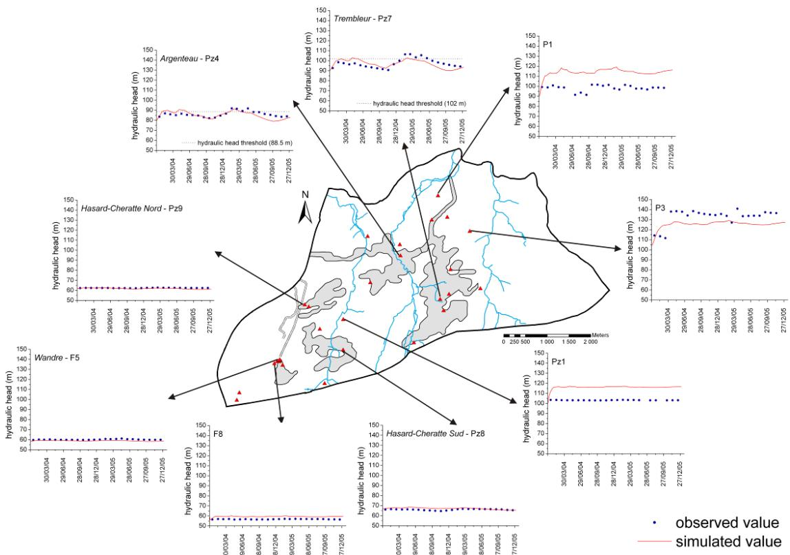
Figure 4. Comparison between observed and simulated hydraulic heads in different piezometers of the case study zone
