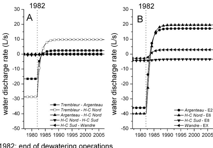
Figure 7. Groundwater rebound scenario - (A) Simulated water discharge rates between exploited zones and (B) Simulated water discharge rates between exploited zones and surface waters
