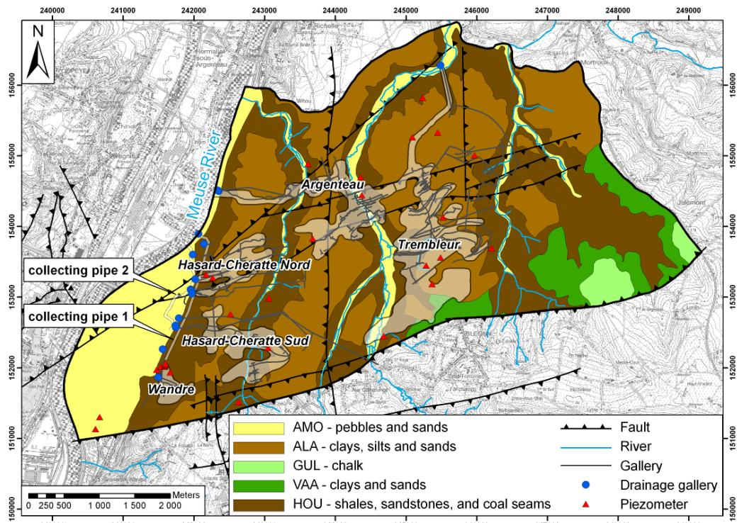
Figure 2. Geological map of the case study zone pointing out the exploited zones
