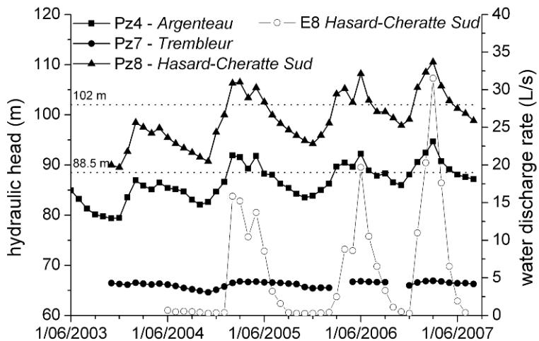
Figure 3. Correlation between hydraulic heads and water discharge rates observed in different networks of galleries (adapted from Dingelstadt et al. (2007))
