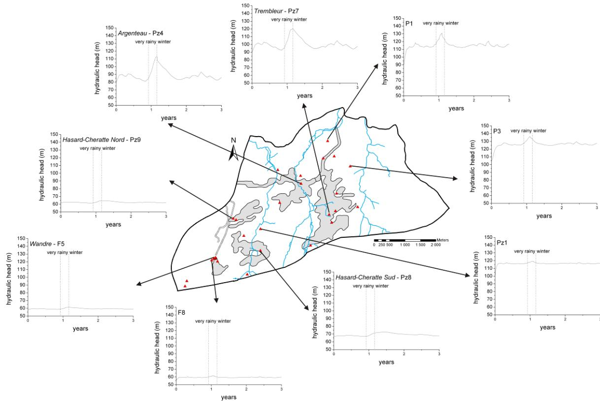
Figure 8. Very rainy winter scenario - Simulated hydraulic heads in different piezometers of the case study zone
