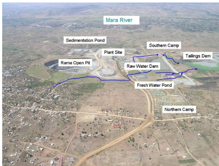
Photograph 2. Some key water management facilities at the Rama area of the North Mara Gold Mine
