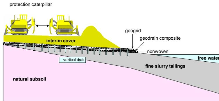
**Figure 2** Installation of vertical drains
