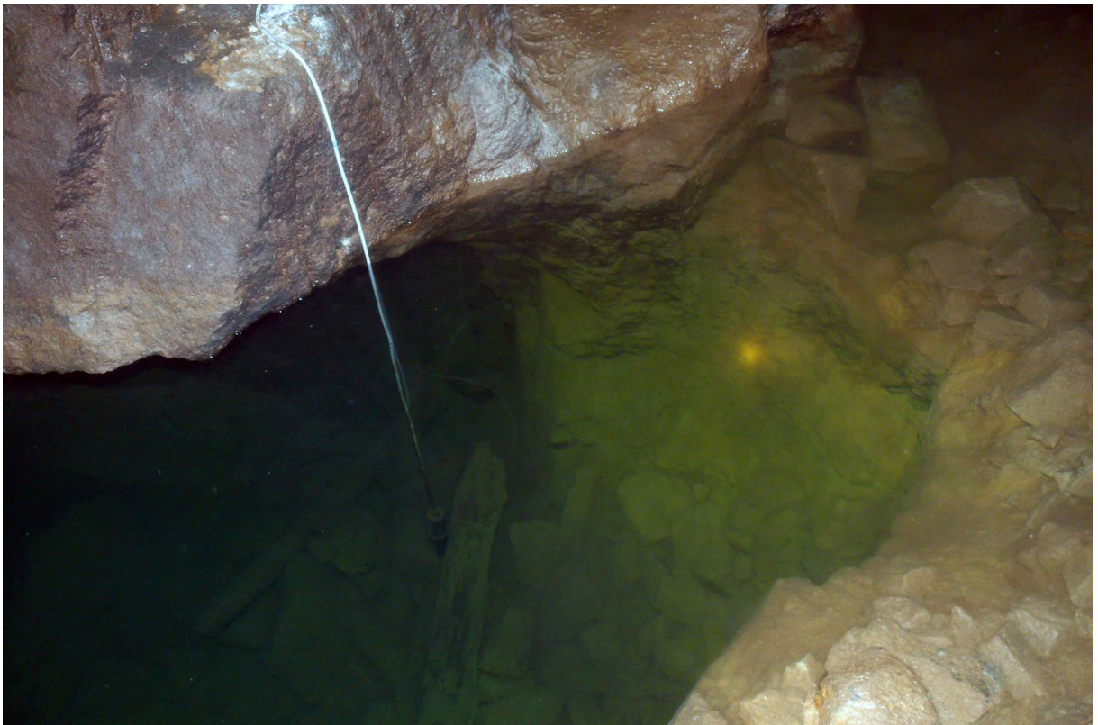
Supplement 4 Probe for continual measurement of fluctuation of mine water level on location V2
