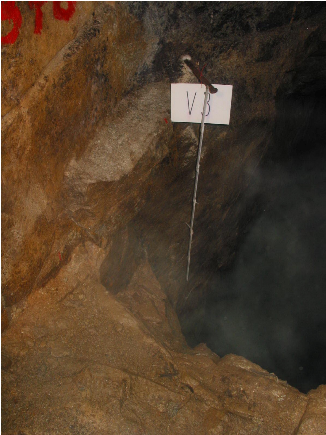
Supplement 6 Sudden loss of water on V3 location in 2003 (fixed meter for quarterly measurements)
