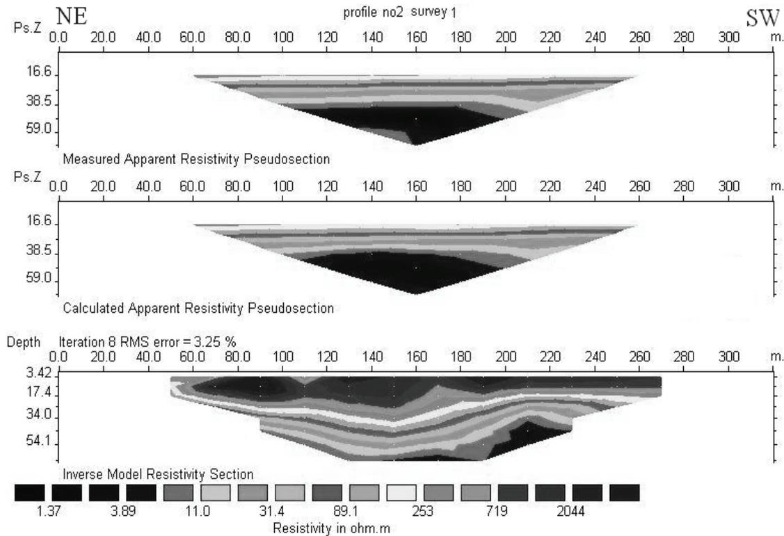
**Figure 3. Inverse modelling results for geoelectrical data indicating measured apparent resistivity pseudosection, calculated apparent resistivity pseudosection and inverse model for profile number 2.**
