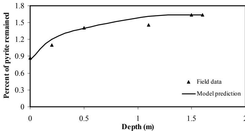
Figure 2. Comparison of the field data and modelling results of the percent of pyrite remained within the waste particles as a function of depth for sample No. 2.
