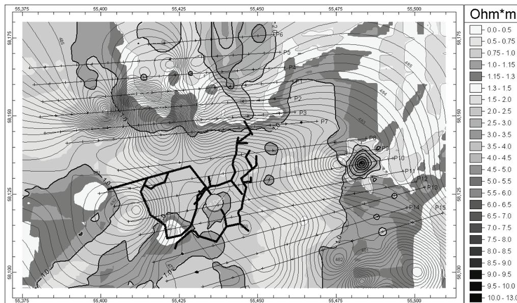
**Figure 8. The horizontal distribution of apparent resistivity at altitude about +480 m.**
