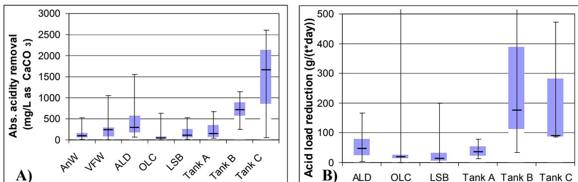
**Figure 7: Box-and-whisker plots of A) absolute acidity removal and B) acid load reduction normalized by system area for the different passive treatment system types (acronyms: see text) published by Ziemkiewicz *et al.* (2003) and for tanks A-C**
