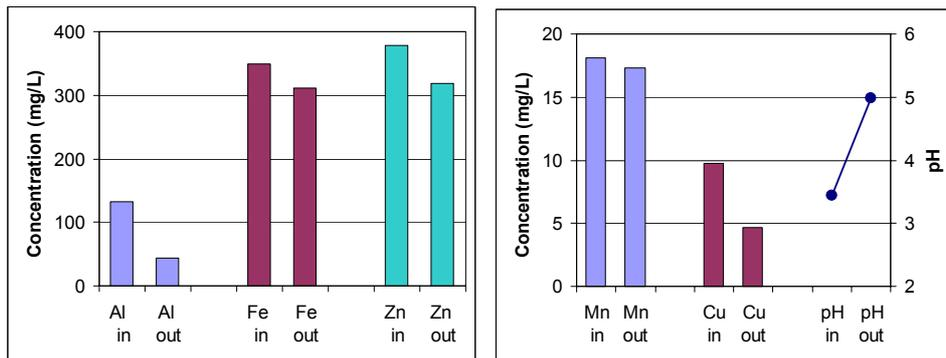
**Figure 4: A) Medians of Al, Fe and Zn concentrations, B) medians of Mn and Cu concentrations (columns) and pH (filled circles) at the in- and outlet of Tank B**
