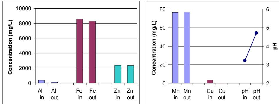
**Figure 6: A) Medians of Al, Fe and Zn concentrations, B) medians of Mn and Cu concentrations (columns) and pH (filled circles) at the in- and outlet of Tank C**
