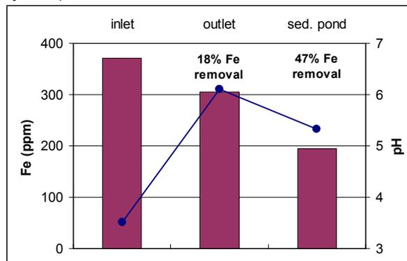
**Figure 5: Effect of the aeration and sedimentation system on Fe elimination: Mean Fe concentrations (columns) and pH (filled circles) at the in- and outlet of Tank B and at the outlet of the sedimentation pond, and Fe removal relative to the inlet concentration**
