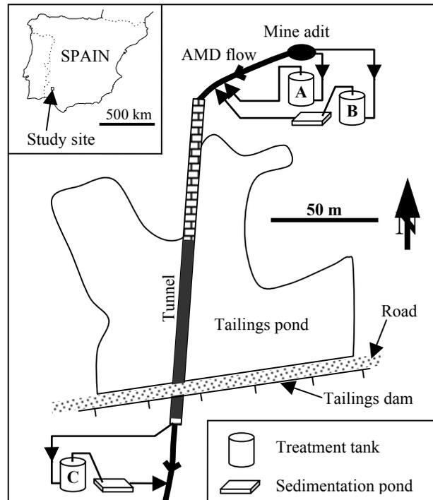
Figure 1: Schematic map of Monte Romero field site and location of experimental treatment tanks
