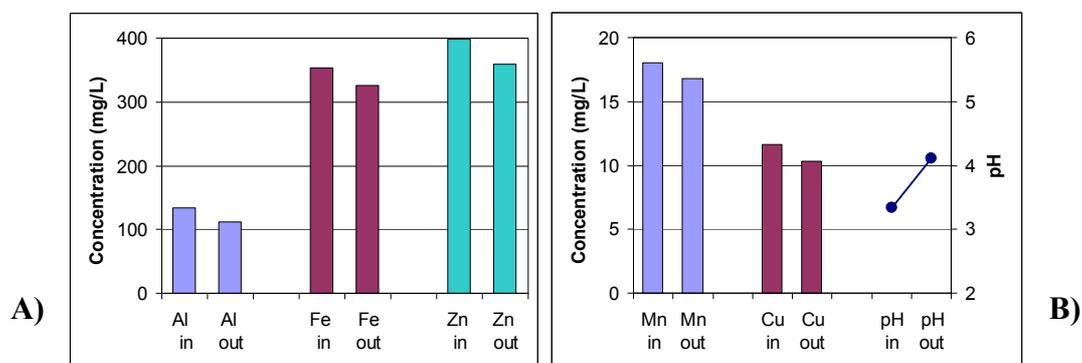
Figure 3: A) Medians of Al, Fe and Zn concentrations, B) medians of Mn and Cu concentrations (columns) and pH (filled circles) at the in- and outlet of Tank A
