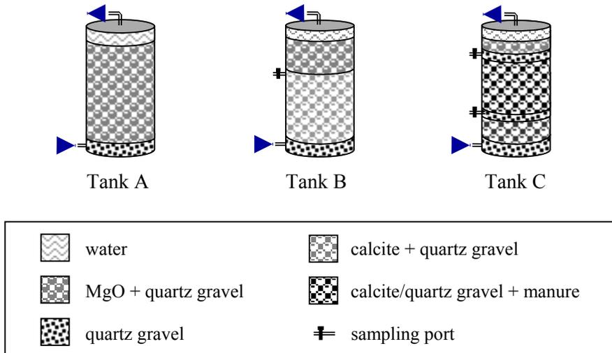
Figure 2: Filling materials of the treatment tanks
