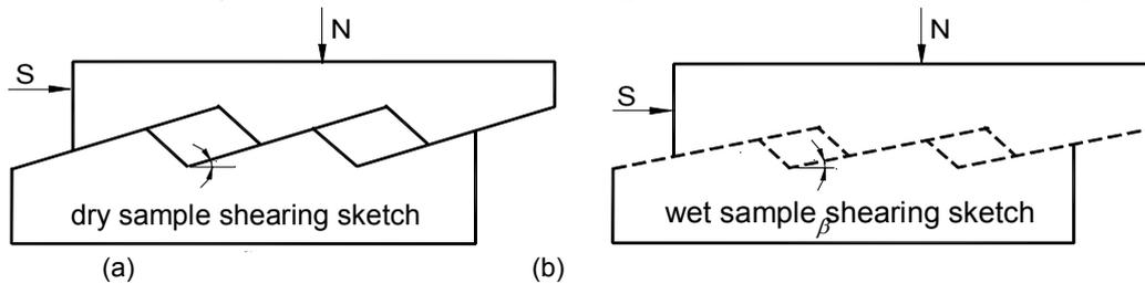
Figure 6. Schematic graph showing the deformation of surface asperities and different sliding surface because of saturation,  $\alpha > \beta$
