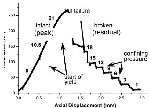
Figure 3: The multistage triaxial compressive testing method
