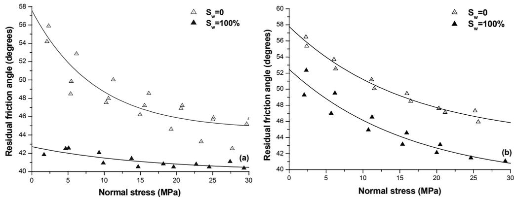
**Figure 5: Developing tendency of the residual friction angle due to water, (a) Coarse grained sandstone (b) Silty sandstone**
