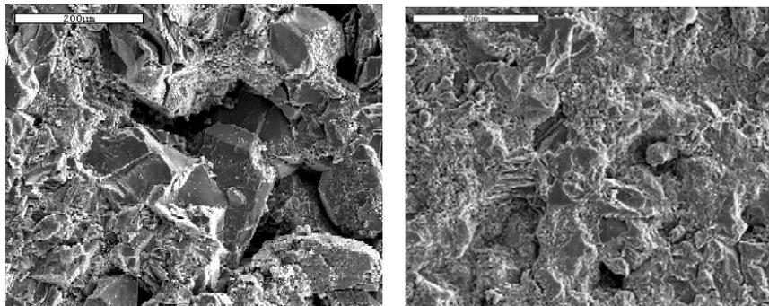
**Figure 1: Topography of Coarse grained sandstone (a) and Silty sandstone (b) from SEM scanning**
