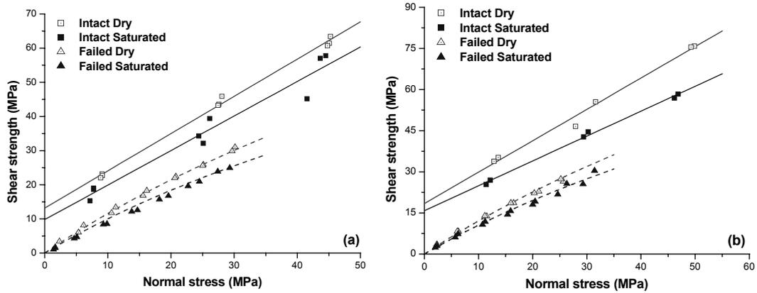
**Figure 4: Strength envelopes of intact and failed (a) Coarse grained sandstone (b) Silty sandstone when dried and saturated**
