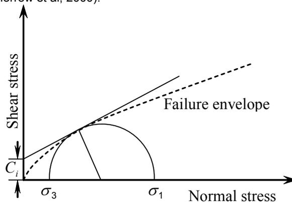
Figure 7: Schematic graph showing the definition of the instantaneous cohesion of rock joint ( $C_i$ ) in terms of axial stress  $\sigma_1$  and confining pressure  $\sigma_3$
