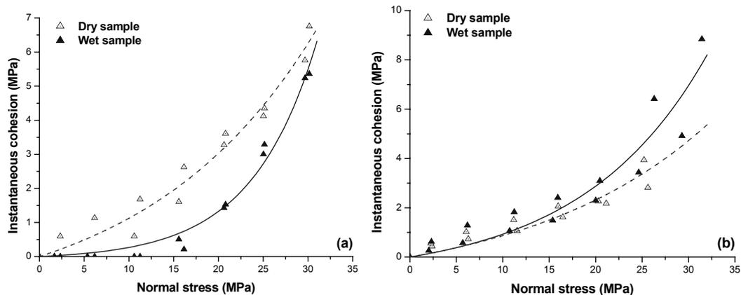
Figure 8: Instantaneous cohesion of the rock joint against the normal stress for (a) Coarse grained sandstone, (b) Silty sandstone
