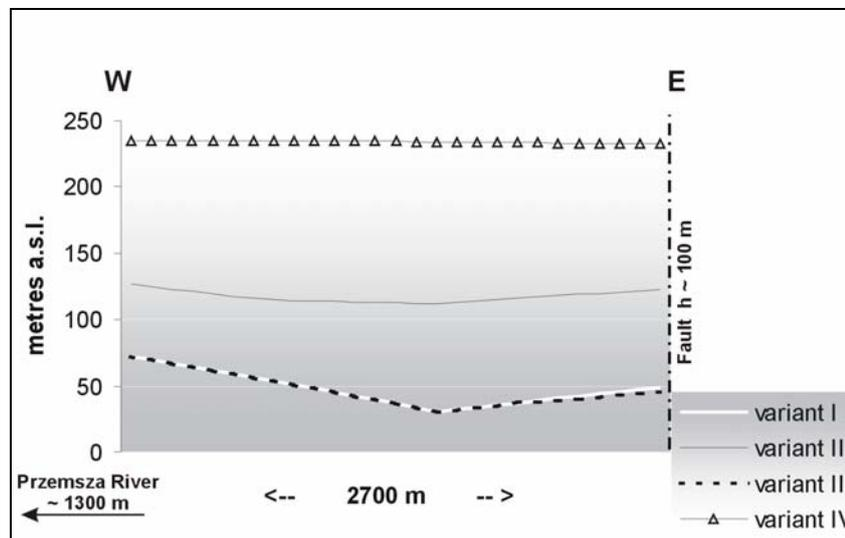
Fig. 2. Hydraulic head across the model area simulated in 4 variants of the model
