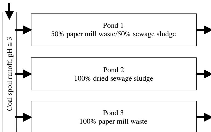
**Fig. 1.** Schematic diagram of the Aspatria pilot-scale wetland site. The arrows show direction of the coal spoil runoff flow. Each pond measures 27 m by 7.5 m (not drawn to scale).
