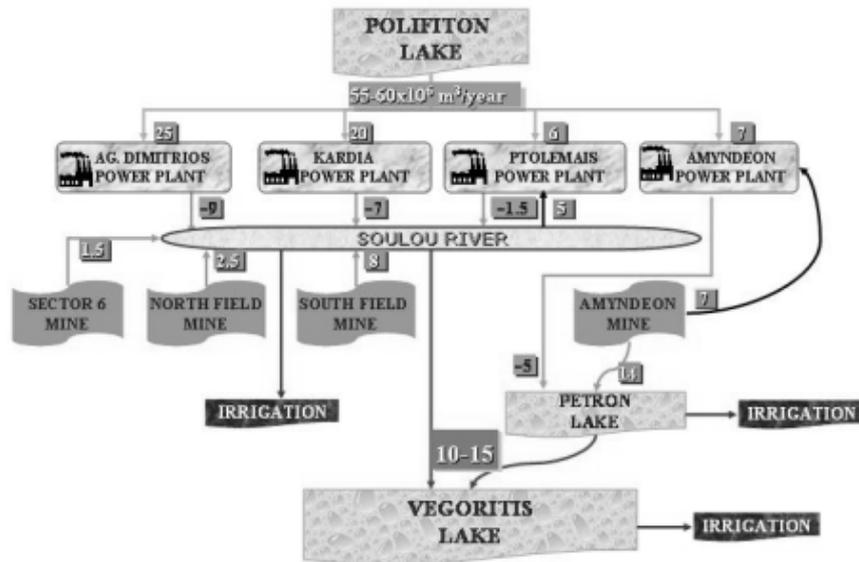
**Fig. 2.** Flow diagram of mining activity and water needs for the year 1996 (all volumes in  $10^6 \text{ m}^3/\text{yr}$ )
