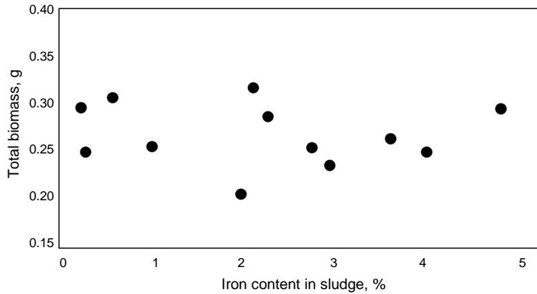
Figure 4. Total biomass as a function of iron content in artificial soil from sand, wood waste and Silwood wetland sludge
