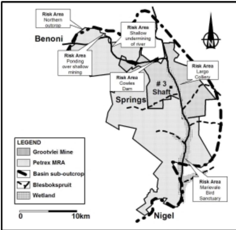
Figure 7 Areas of high risk for infiltration of surface water to the mines
