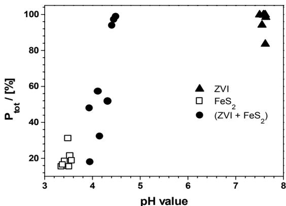
**Fig. 3.** Comparison of the total fixation rate as function of the final pH value for the three experimental systems.
