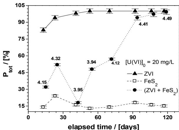
**Fig. 1.** Uranium fixation by zero valent iron (ZVI: 15 g/L), a pyrite mineral ( $FeS_2$ : 25 g/L) and the mixture of both materials (ZVI +  $FeS_2$ ) as a function of the time. The reported numbers on the plot (ZVI +  $FeS_2$ ) are the corresponding final pH values. The lines are given to facilitate visualization.
