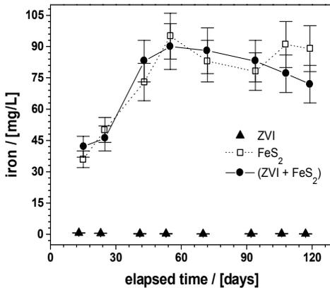
**Fig. 2.** Variation of the iron concentration in the experimental systems with the time. The represented lines are not fitting functions, they just joint the point to facilitate visualization. The big errors in system II & III resulted from the strong dilution (1/100).
