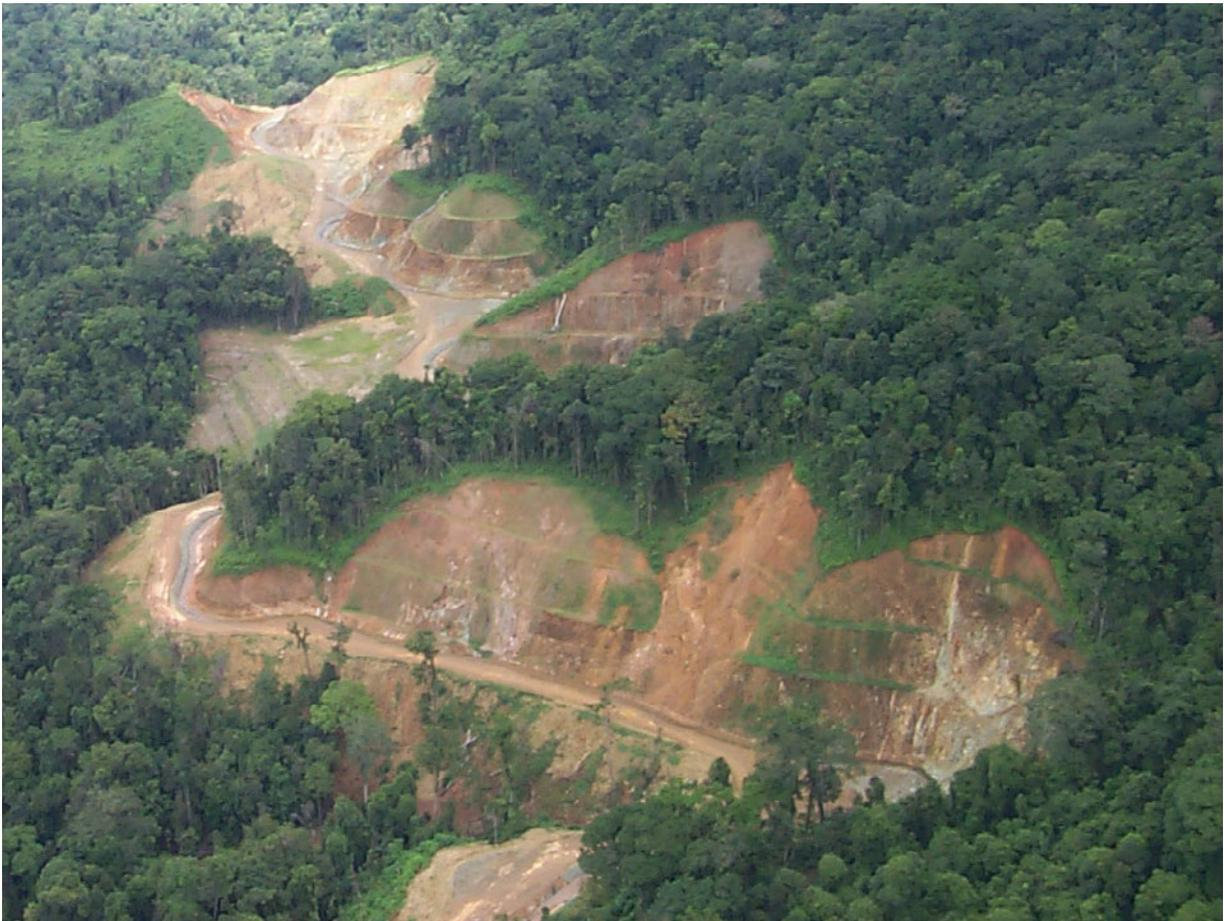
Photo 3: Channel with moderate slopes and no side cast.
