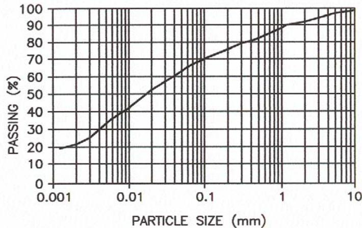
Figure 1: Gradation of Typical Surficial Soils
