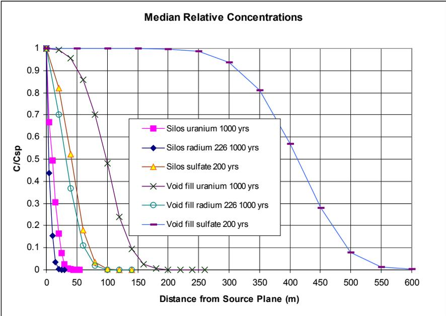
Figure 4 Monte Carlo simulations of relative concentrations of uranium after 1000 years from silos in an easterly direction.
