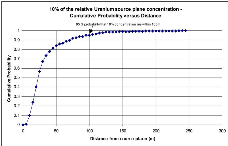
Figure 6 Cumulative probability of the 10% uranium relative concentration versus travel distance
