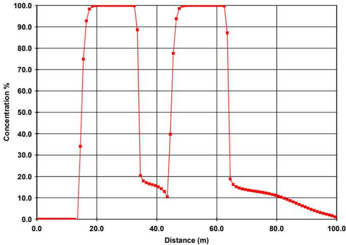
Figure 3 1000 year relative uranium concentration profile through two silos – groundwater flow from left to right.
