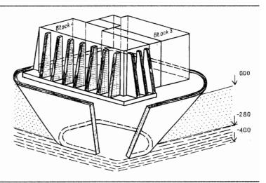
Figure 2. Encasement of the block 3 &4 of the Chernobyl NPP.
