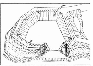
Figure 1. Arrangement of grout holes around tailing pond No. 1 of the Nicopol Ferroalloy Fat
