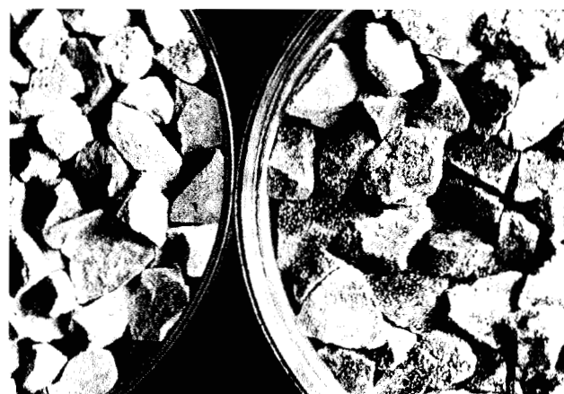
Figure 4. A mineral ore triturated to 1/4 inch, comprising chalcocite as the predominant specimen of copper, not subjected (left) and subjected (right) to biooxidation in dry conditions.
