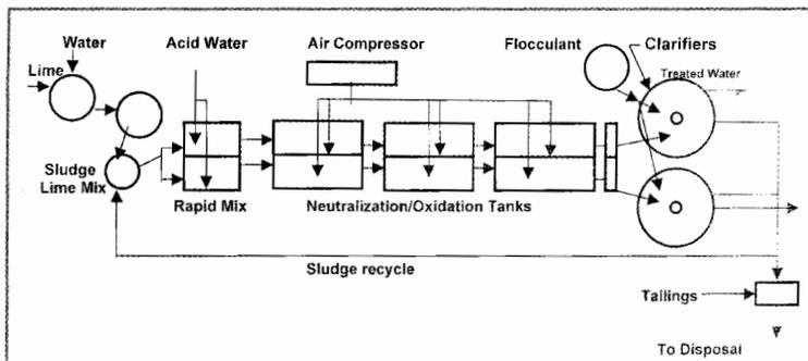
Figure 4. Boliden Apirsa HDS lime neutralization treatment plant.
