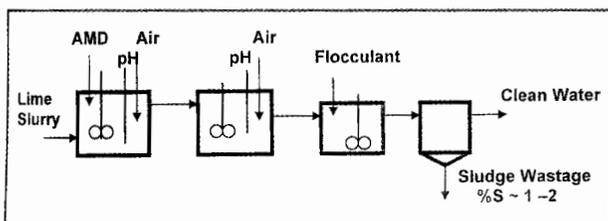
Figure 2. Lime addition to neutralization reactors: Basic-Conventional Method.
