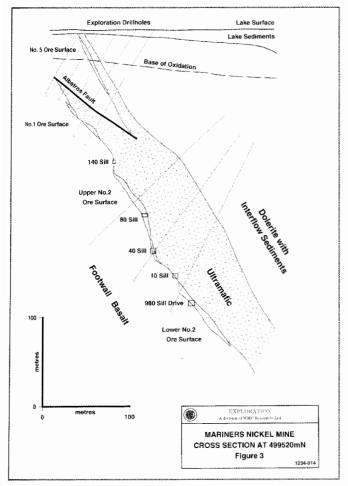
Figure 3. Cross section.
