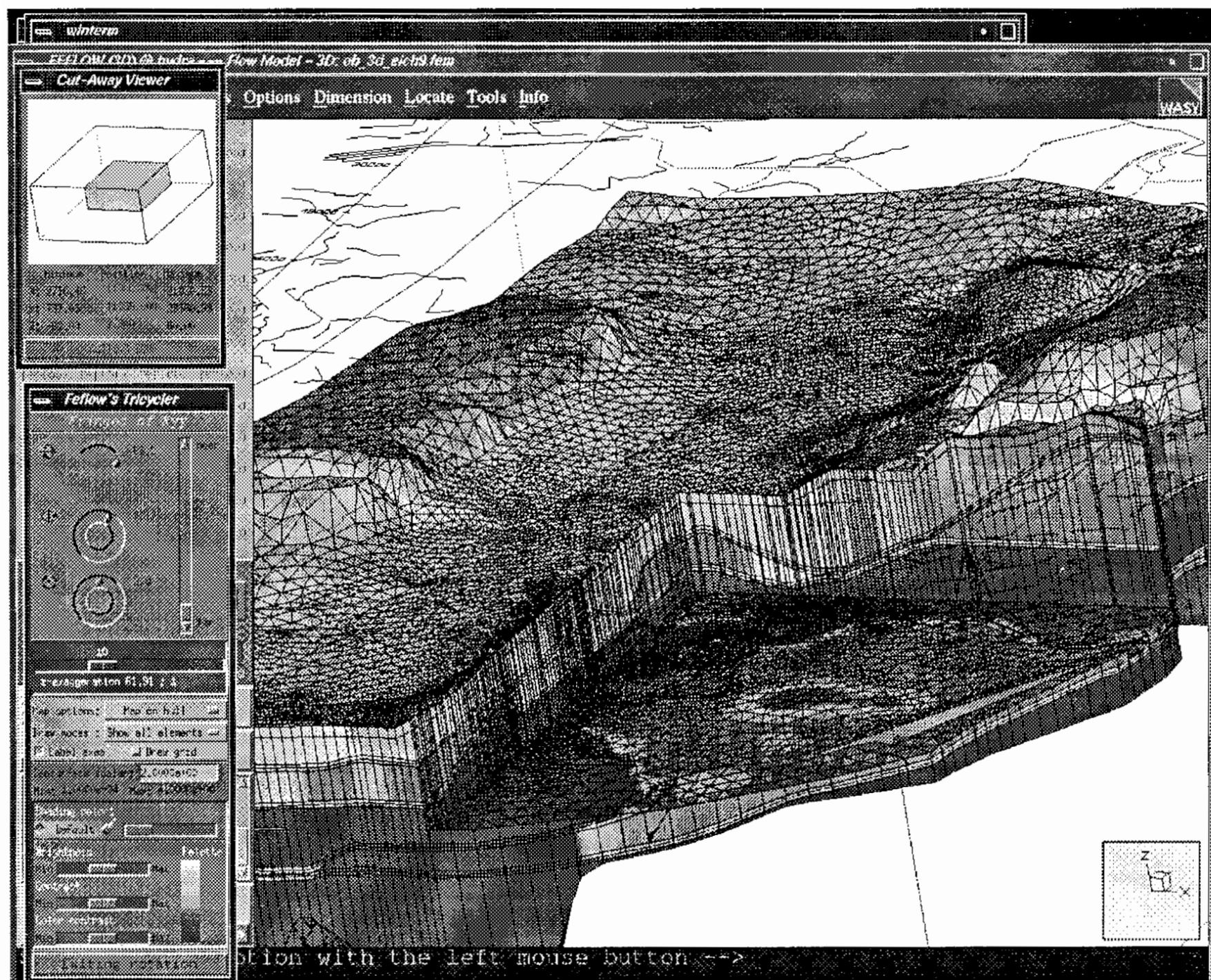
Figure 2: FEFLOW-3D: model for a multi-layer aquifer system
