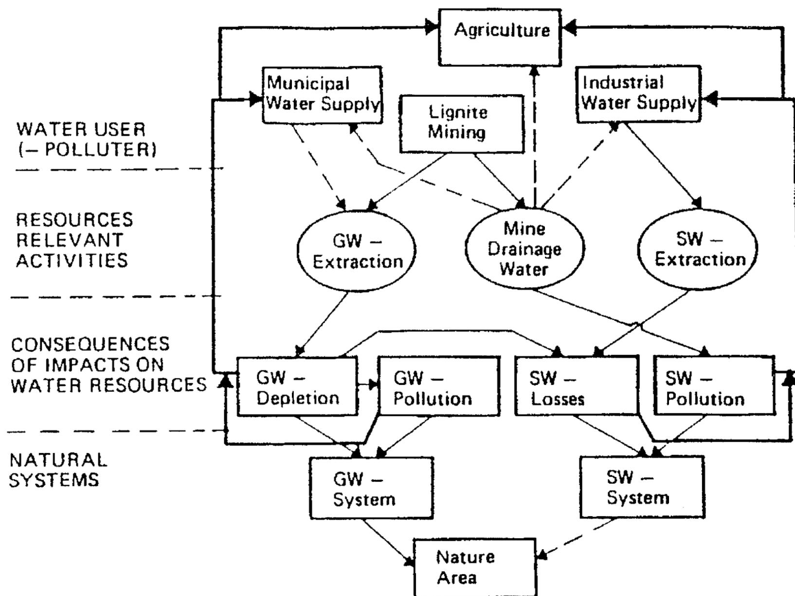
Figure 3: Impact diagram for open-pit lignite mining
