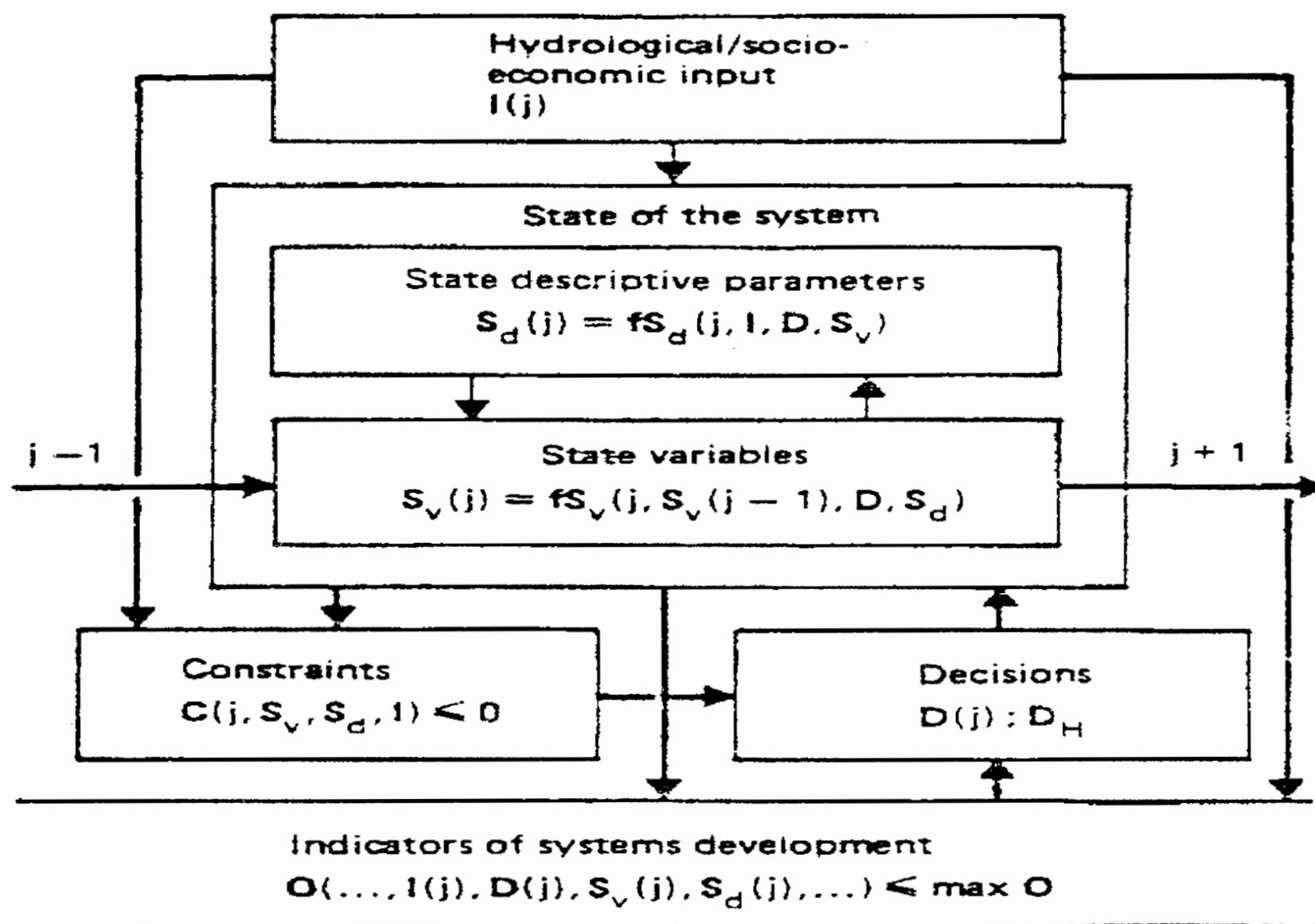
Figure 4: Block schema of the planning model, DSS MINE
