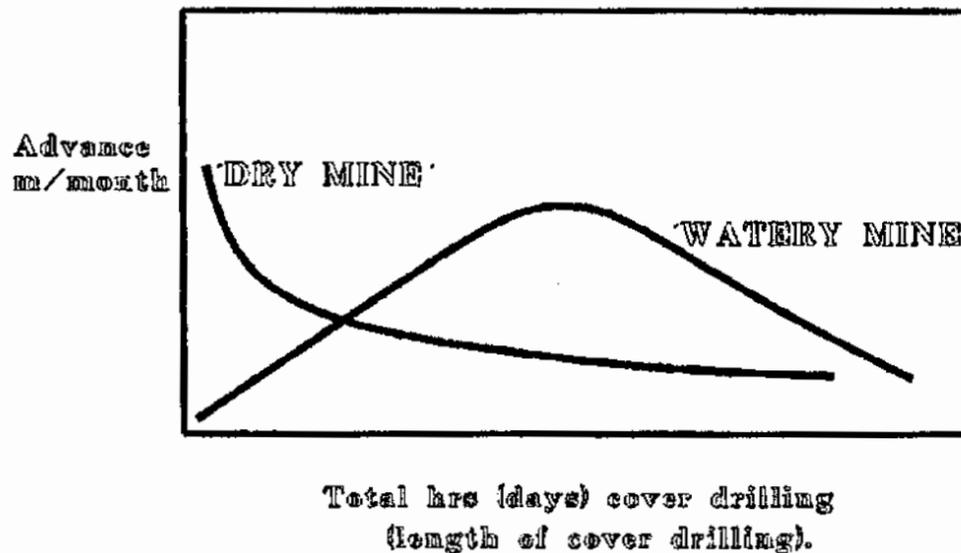
FIGURE - 7 : Mining advance against time spent on cover drilling and grouting.
