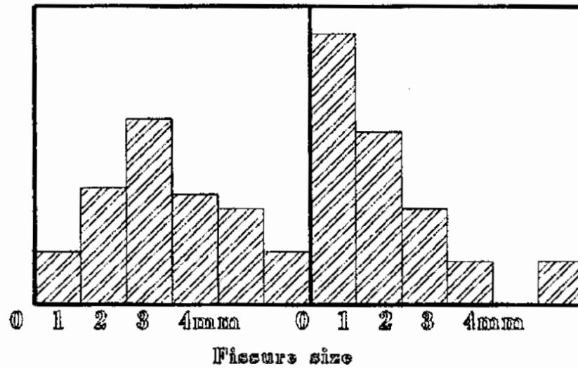
FIGURE - 6 : Possible fissure sizes and frequencies for typical cover grouting and drilling.
