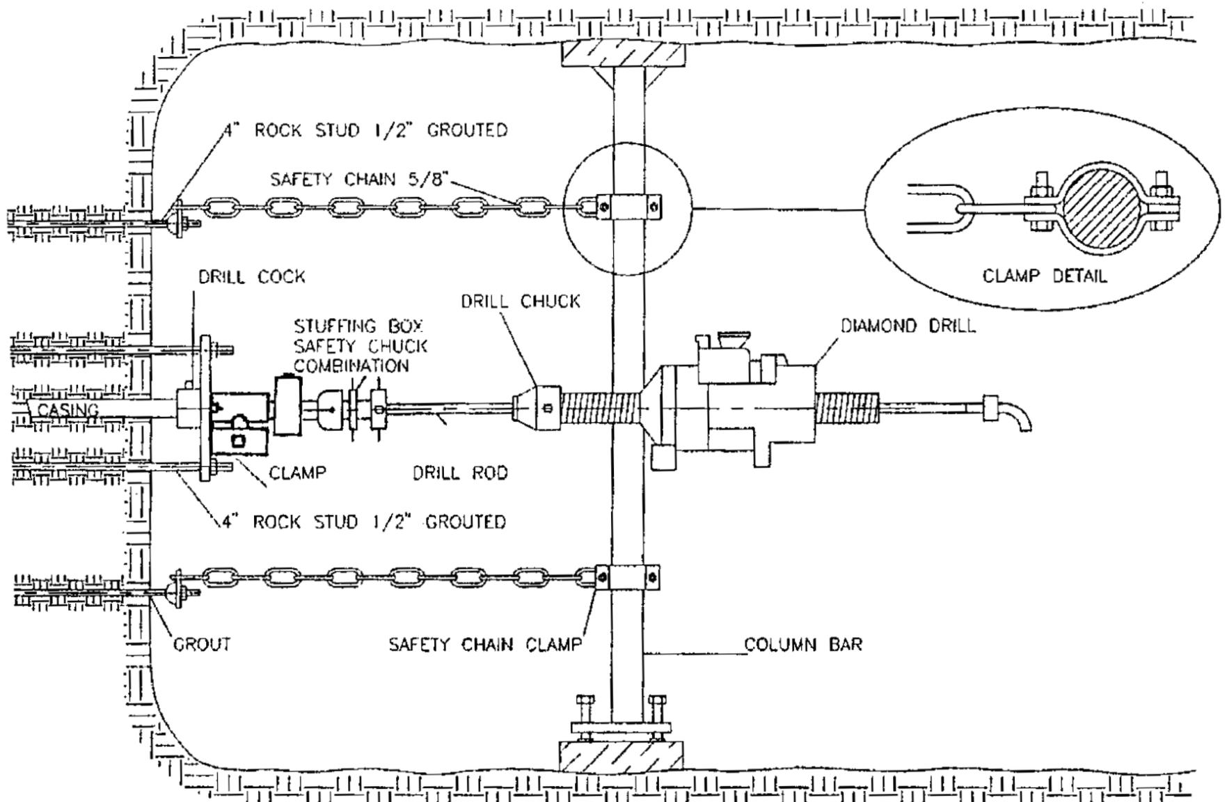
Drawing 1: Schematic presentation showing High Pressure Safety Valves configuration for High Pressure Drilling
