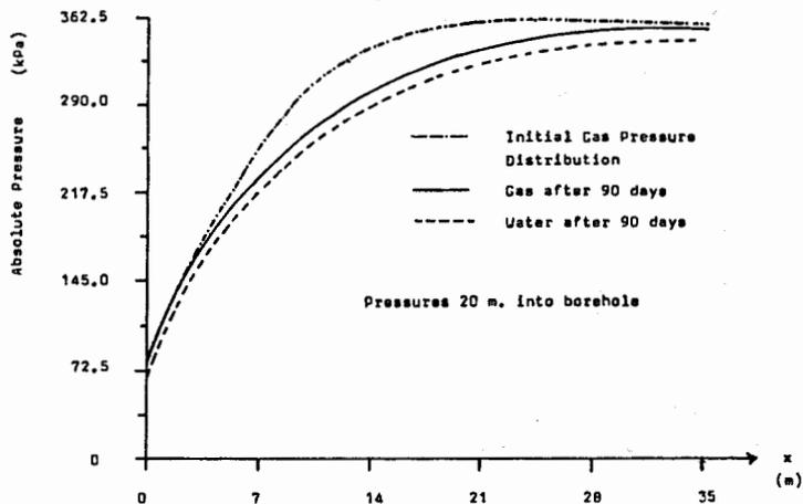
Figure 8 Calculated pressure Prediction of gas and water for multiple boreholes using Darcy's Law (90 days)
