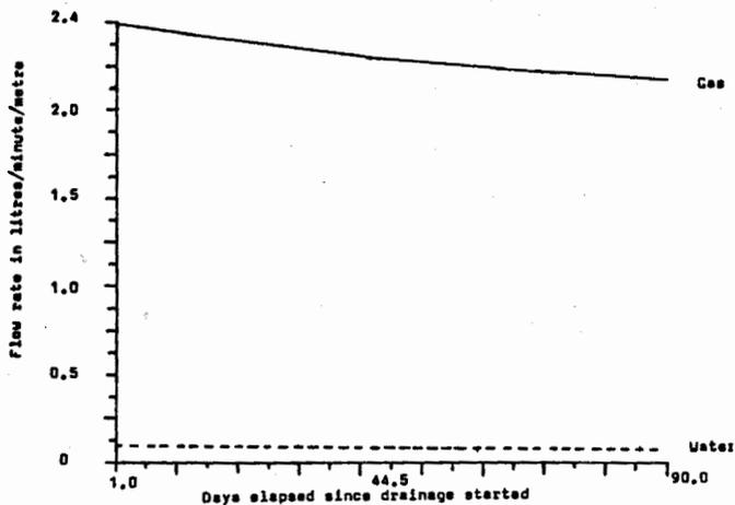
Figure 11 Calculated flow rates of gas and water per metre of borehole length (90 day period)
