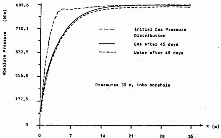
Figure 9 Calculated prediction of gas and water pressure 45 days after drainage commences (20m borehole)
