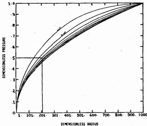
Figure 1 Prediction of gas pressure drop in coal seams against radial distance using Darcy's equation.
