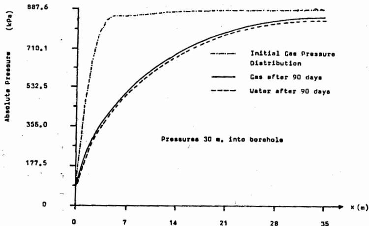
Figure 10 Calculated gas and water pressure distributions 90 days after drainage commences (30m borehole)
