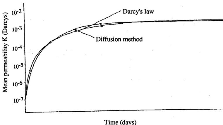
Figure 3 Comparison of Darcy's method and diffusion method for the calculation of permeability
