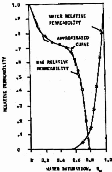
Figure 5 Relative permeability of gas and water vs water saturation
