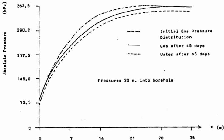
Figure 7 Calculated pressure prediction of gas and water for multiple boreholes using Darcy's Law (45 days)
