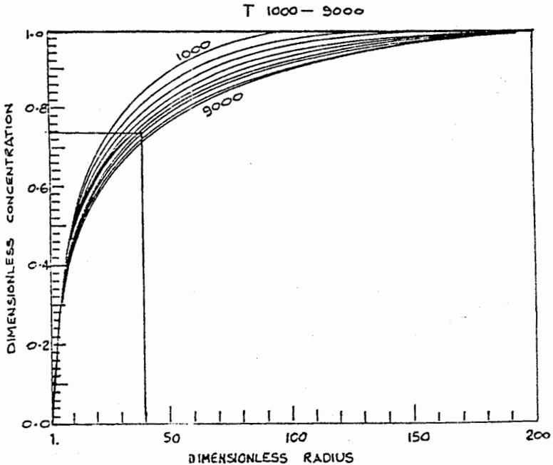
Figure 2 Prediction of gas concentration with radial distance using Fick's Law
