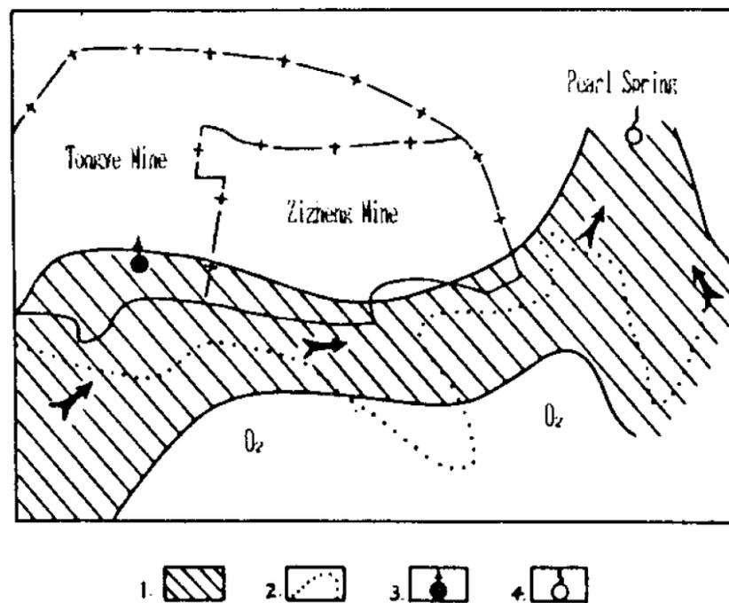
1. O<sub>2</sub> Runoff Zone, 2. O<sub>2</sub> Boundary Line, 3. Collapse Column Water Inrush Site, 4. O<sub>2</sub> Spring
