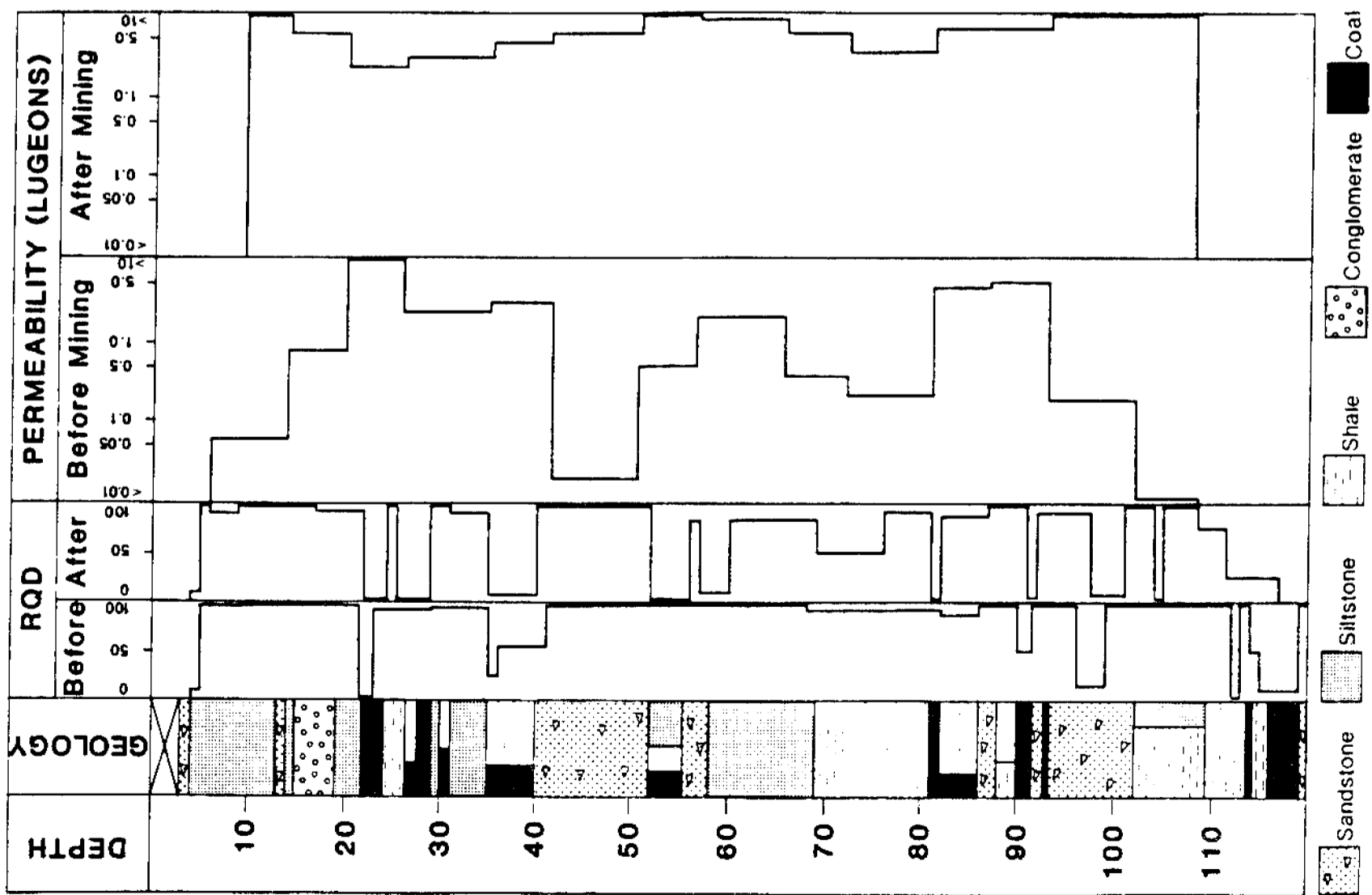
FIGURE 5 - Changes in bulk permeability and RQD - Invincible Borehole
