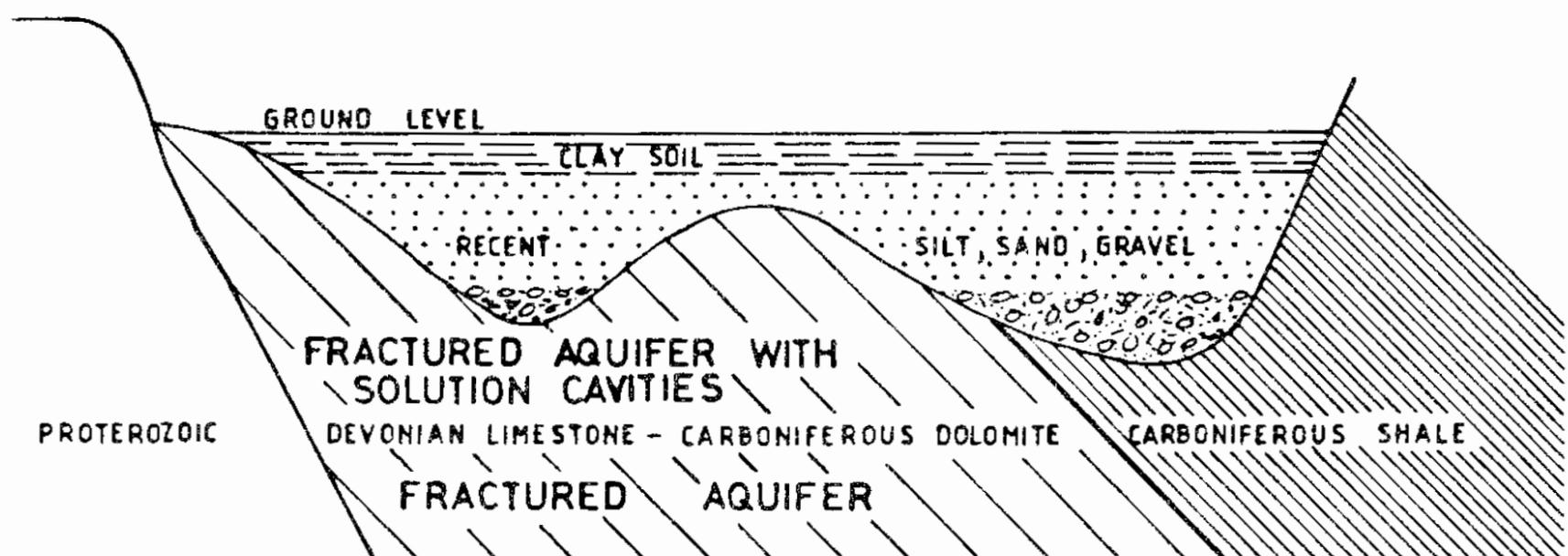
Figure 1. Diagrammatic cross-section through aquifer.
