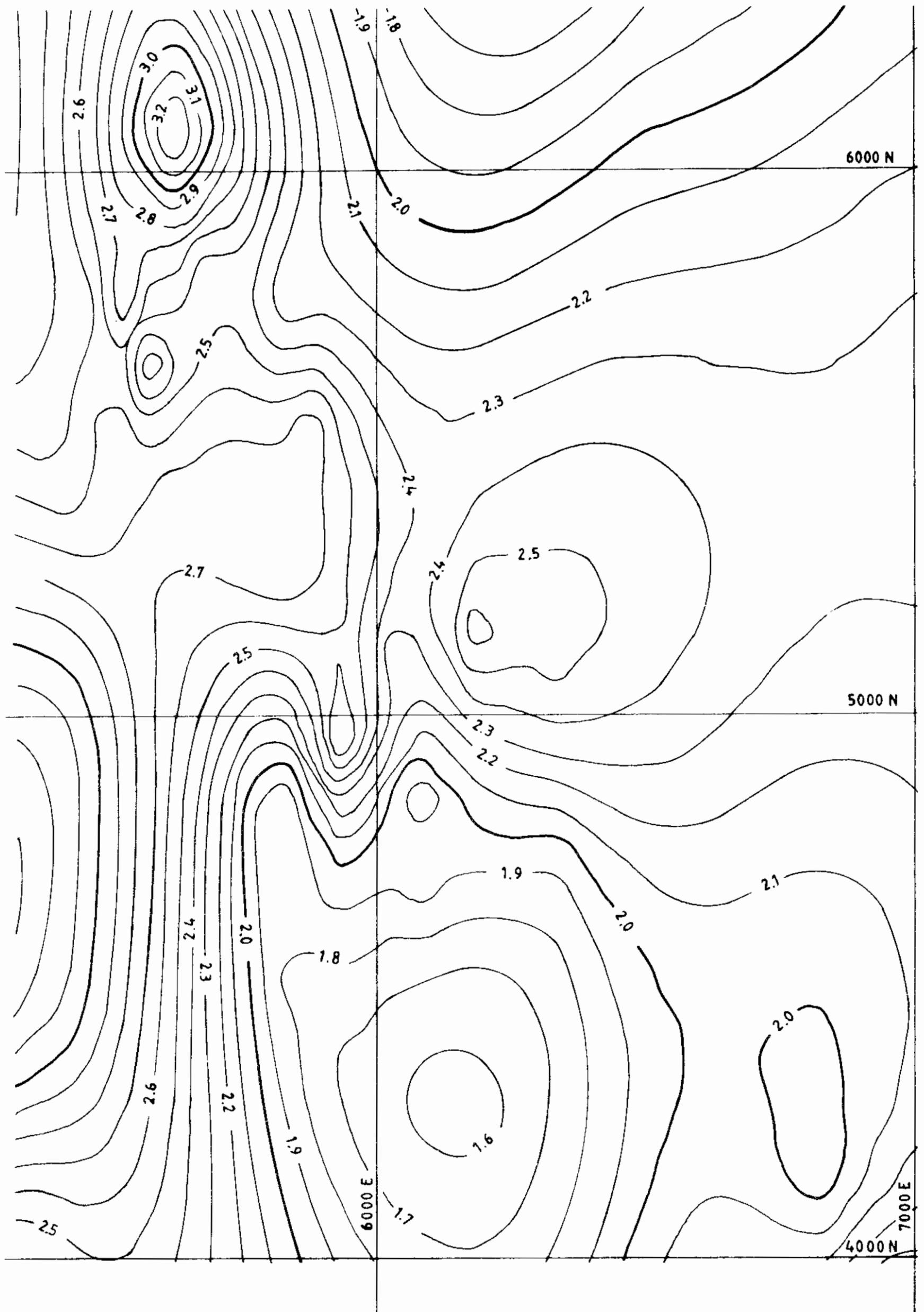
Figure 4. Total fracturation index for Area 2.
