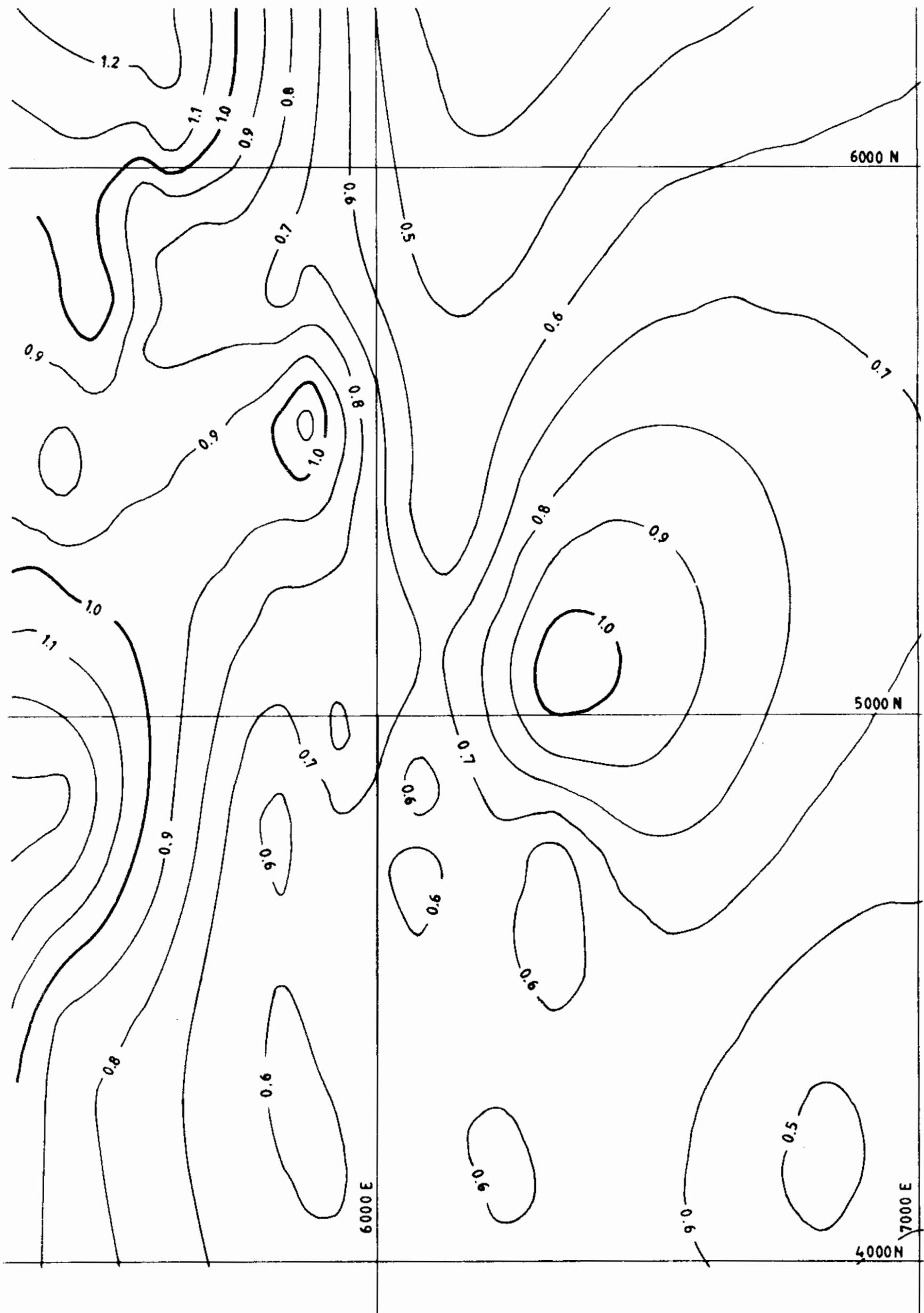
Figure 5. Effective opening fracturation index for Area 2.
