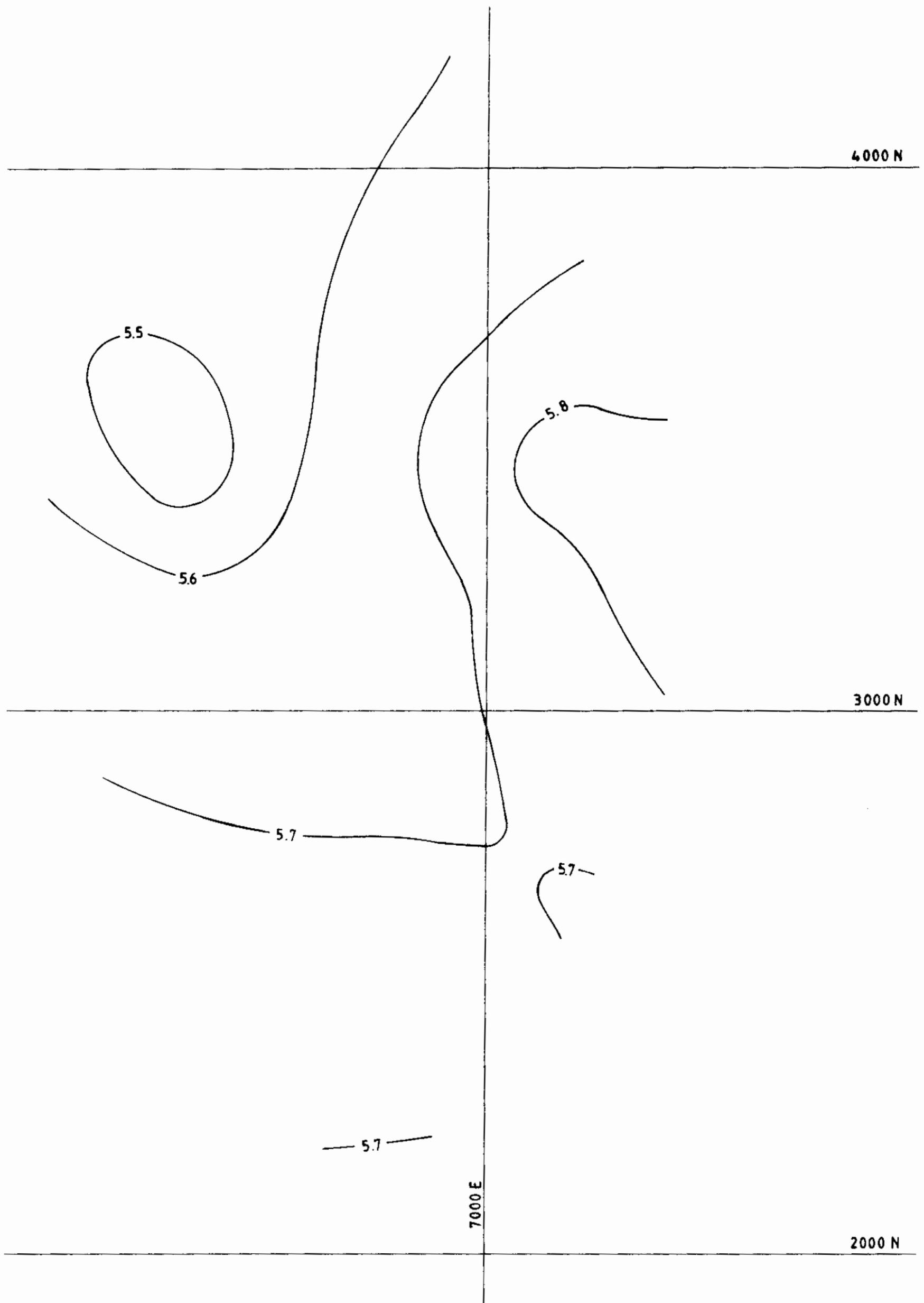
Figure 6. Pre-pumping piezometric surface for Area 1.
