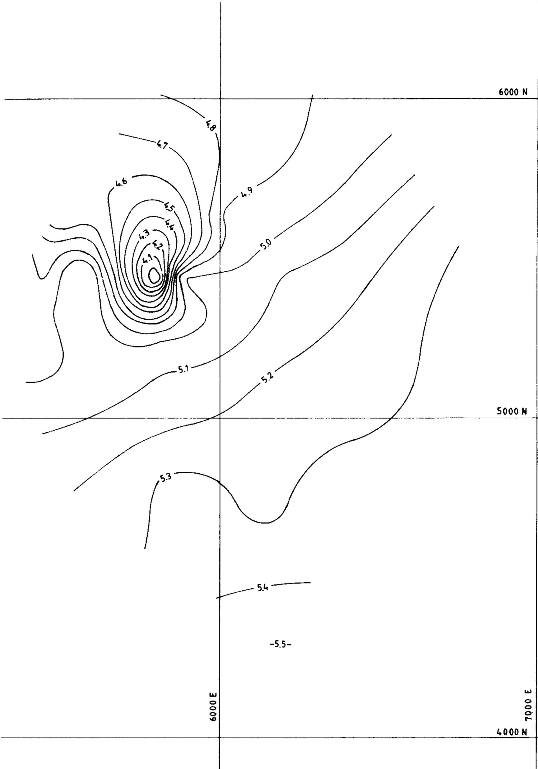
Figure 9. Maximum drawdown piezometric surface for Area 2.
