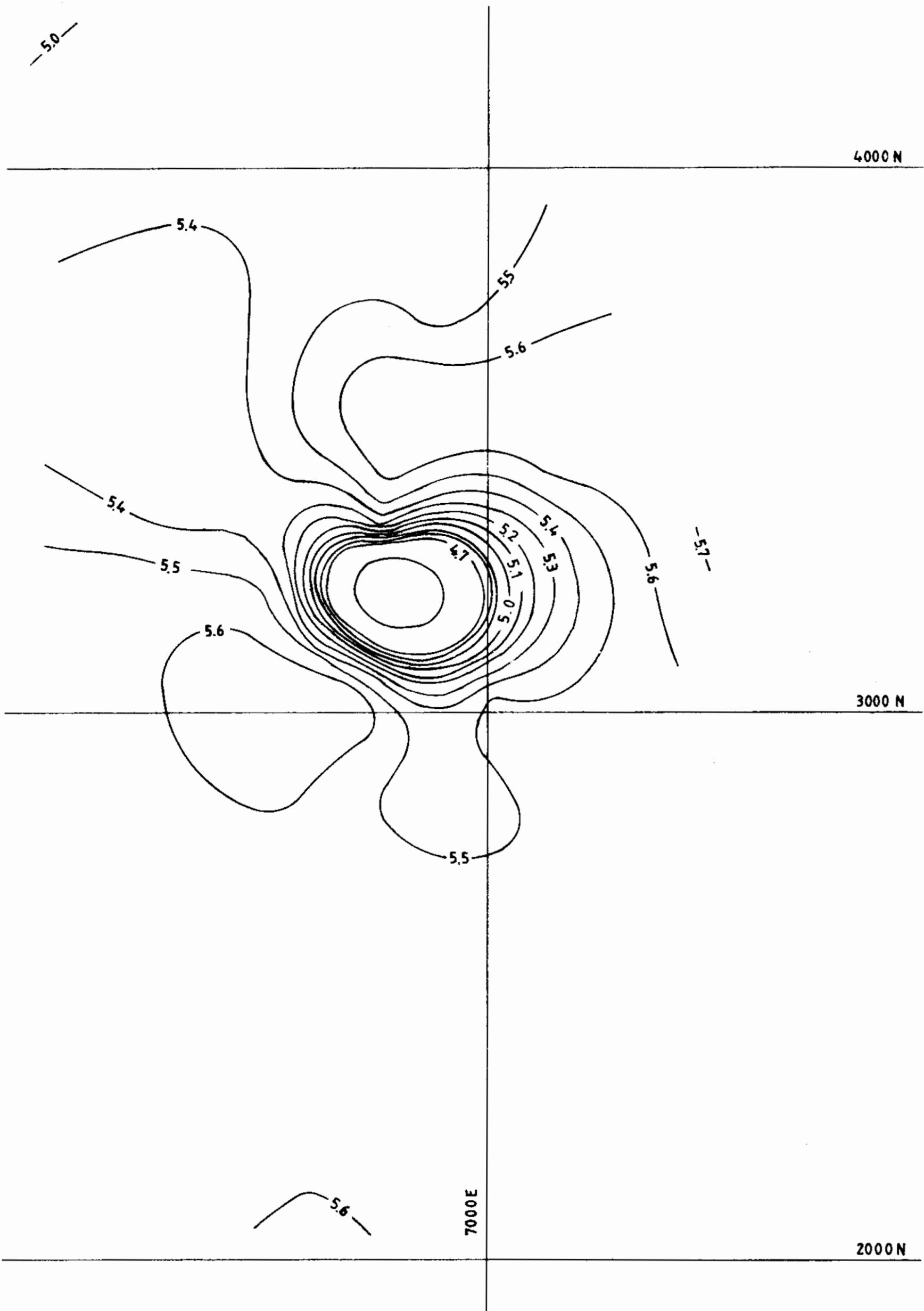
Figure 7. Maximum drawdown piezometric surface for Area 1.
