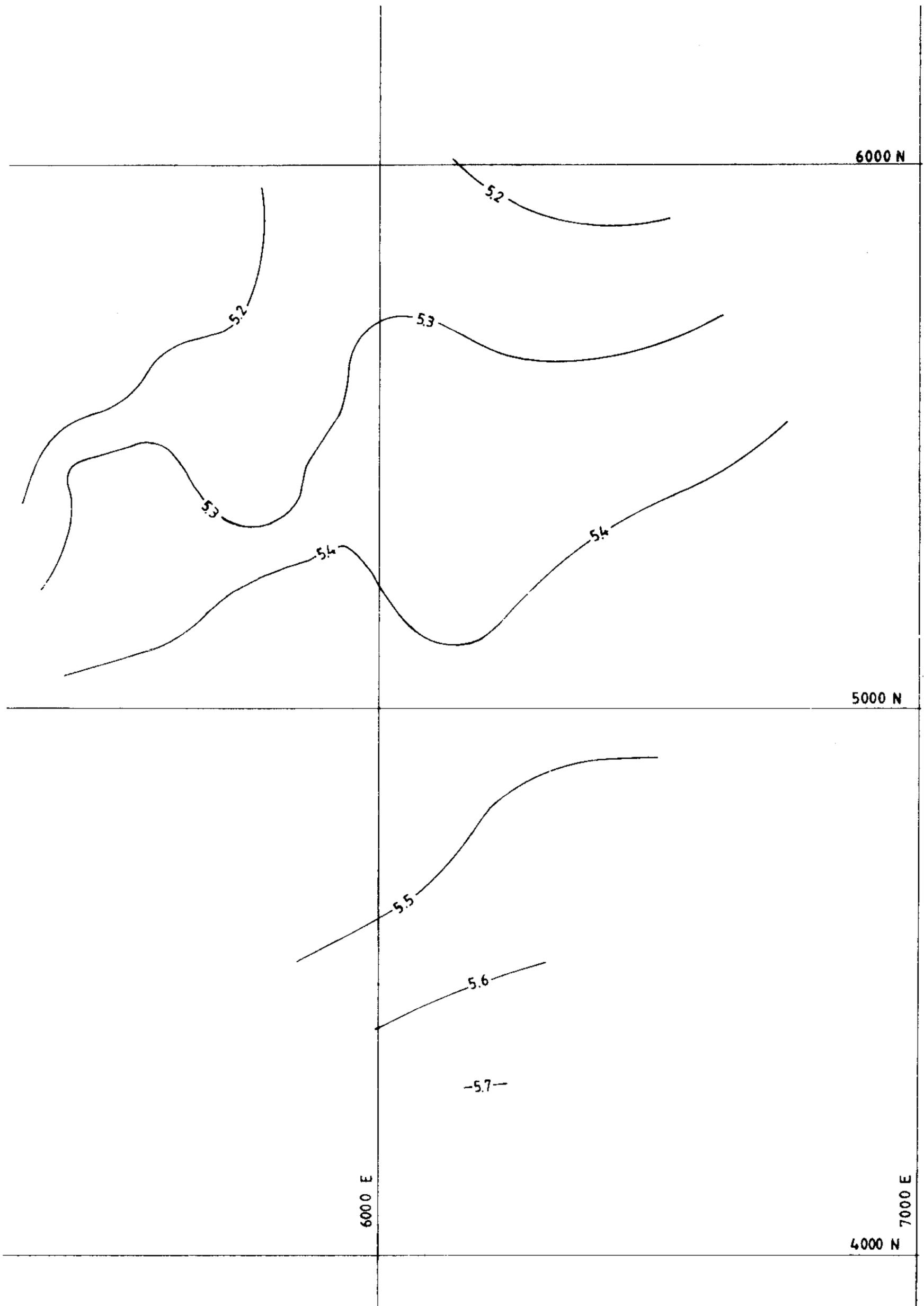
Figure 8. Pre-pumping piezometric surface for Area 2.
