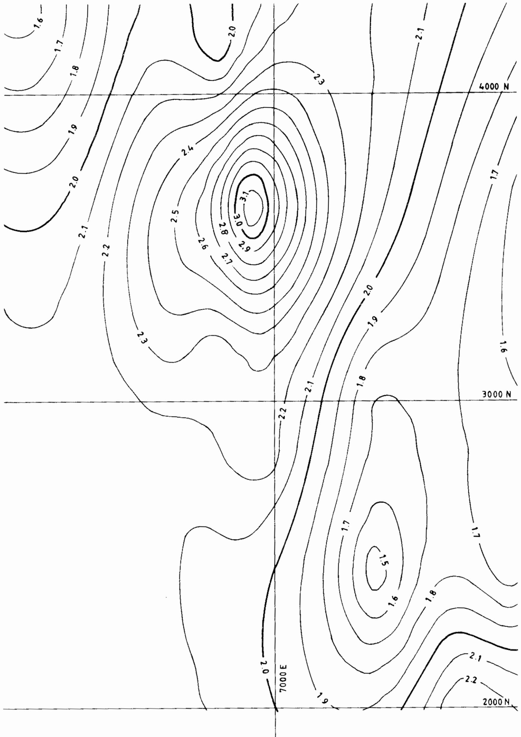
Figure 2. Total fracturation index for Area 1.
