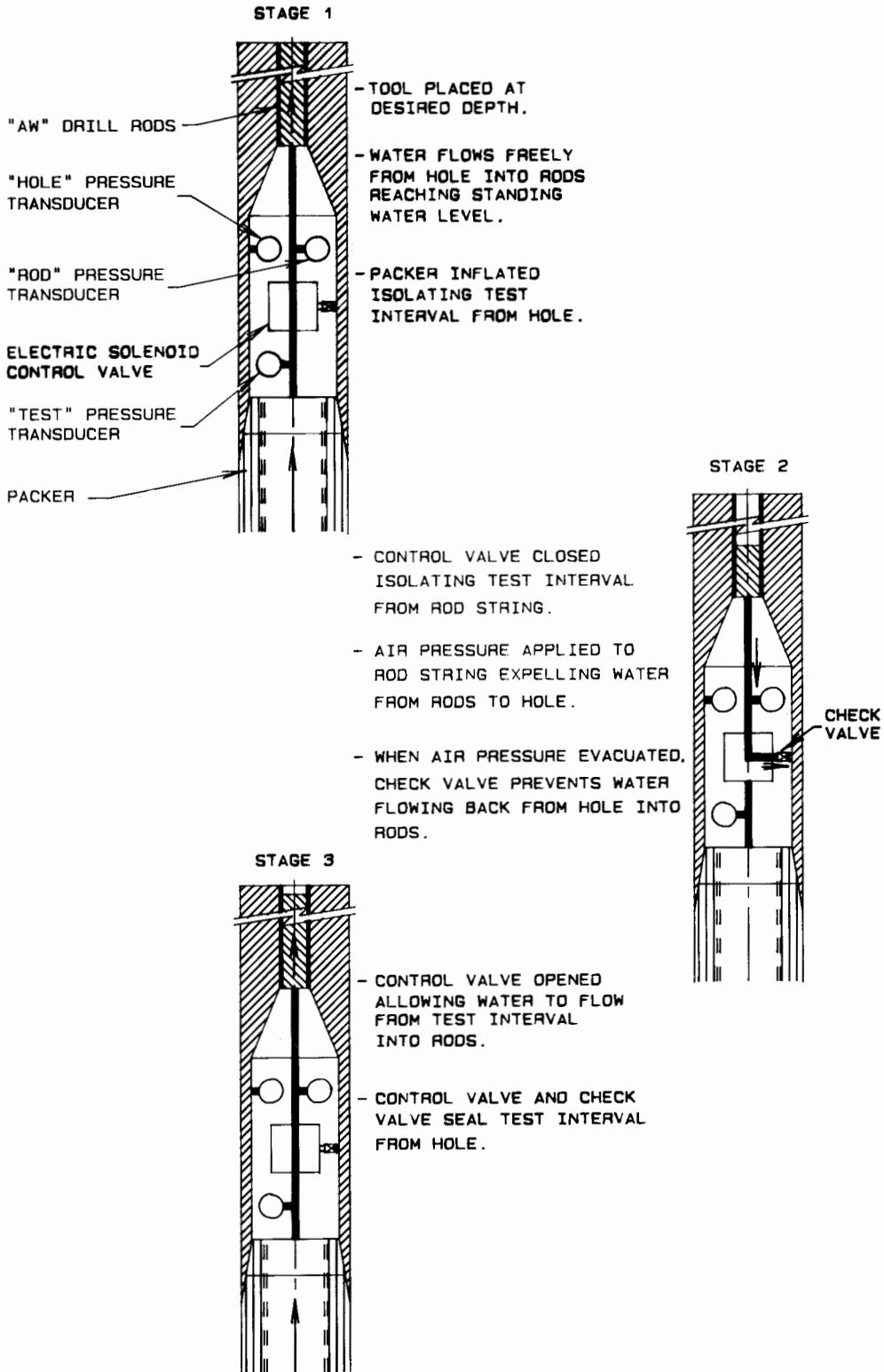
Fig.2. Principle of operation for production test
