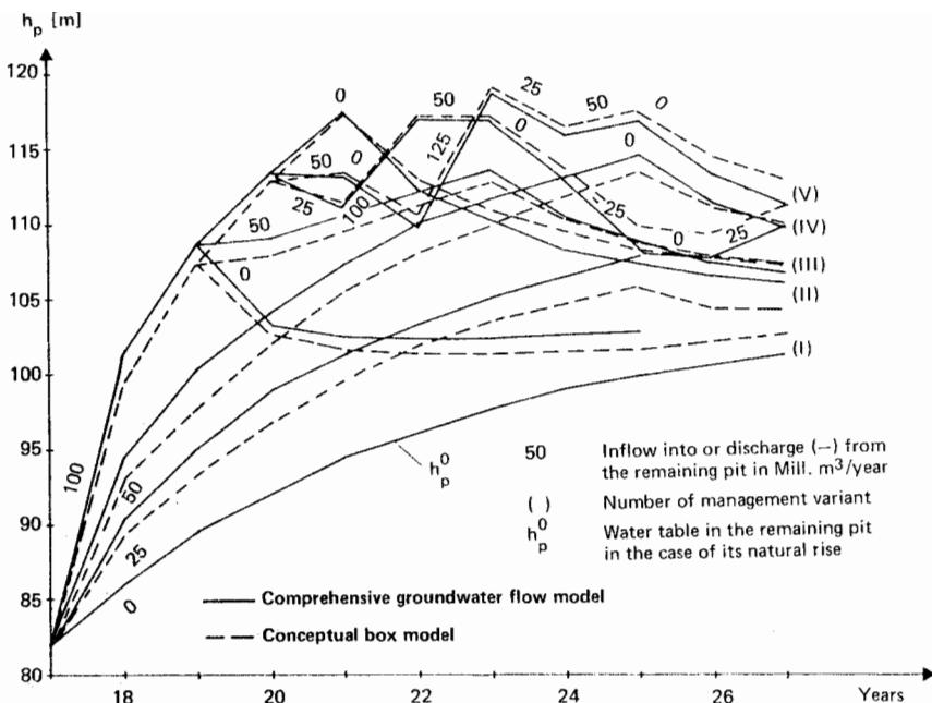
Figure 6: Water table in the remaining pit for different management variants - conceptual box-model
