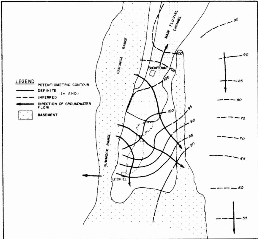
FIGURE 4- GROUNDWATER FLOW AND RECHARGE SYSTEM
