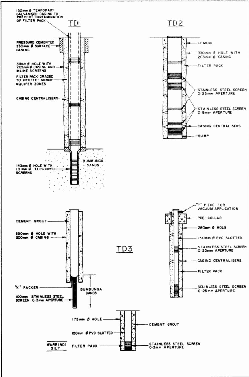
FIGURE 6- DEPRESSURISATION BORE CONSTRUCTION DETAILS
