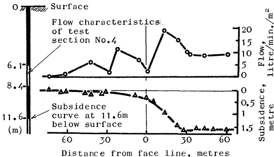
Figure 14. Flow characteristics of test section No. 4 in relation to sub-surface subsidence arising from undermining, Wentworth instrumented borehole
