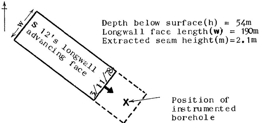
Figure 10. Location of instrumented borehole in relation to longwall face position (Wentworth site)
