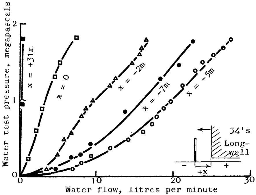
Figure 6. Borehole No.3 flow characteristics
