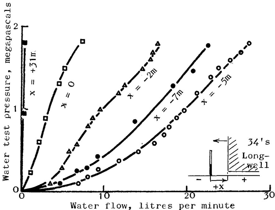
Figure 6. Borehole No.3 flow characteristics
