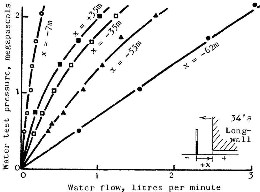
Figure 7. Borehole No.5 flow characteristics.
