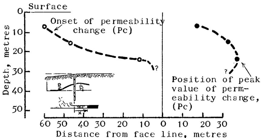
Figure 16. Position of onset and peak value of permeability change of strata overlying a longwall extraction due to undermining
