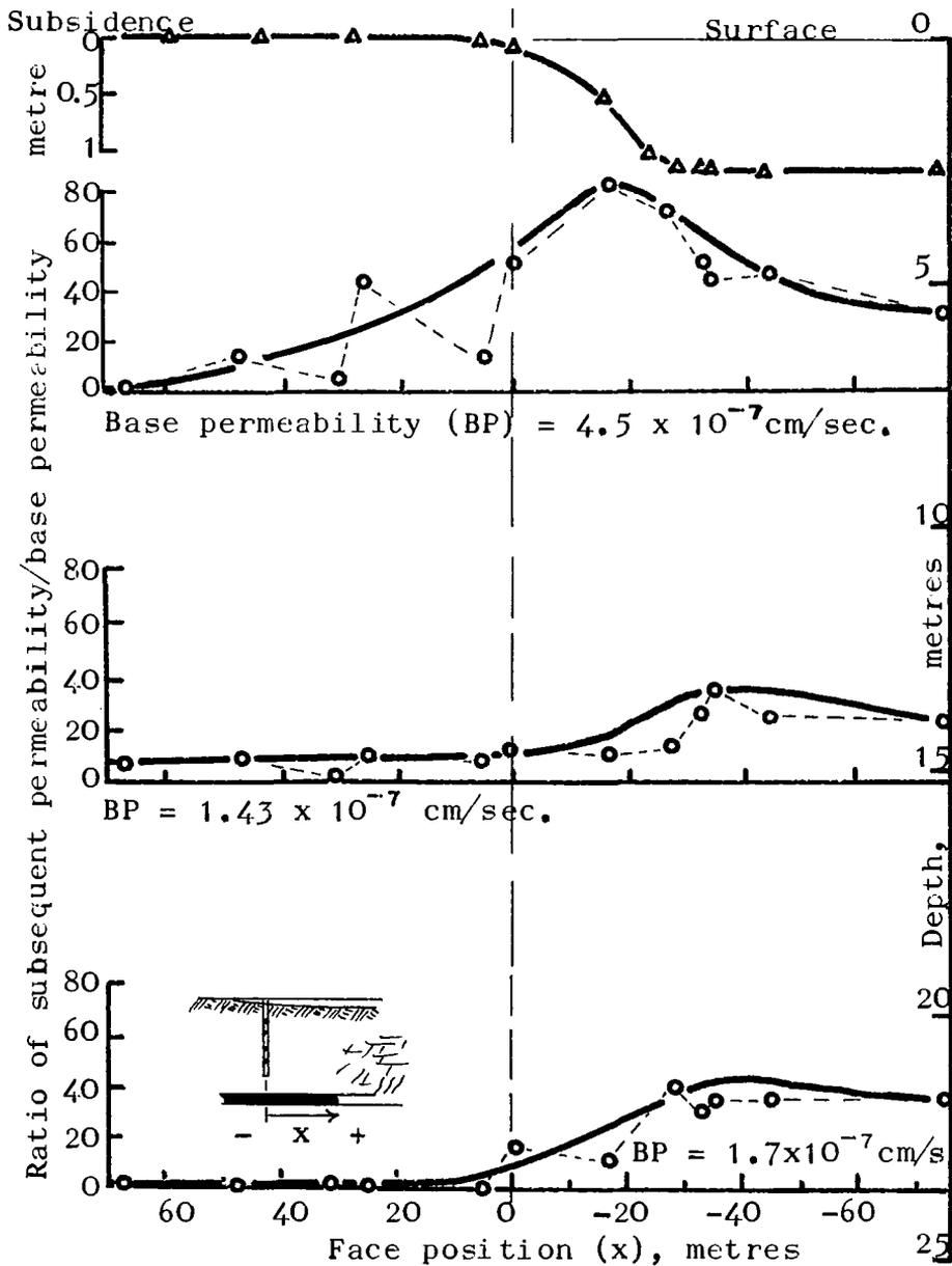
Figure 15. Illustrating comparison of change in ground permeability of strata overlying a longwall extraction (Wentworth instrumented borehole)
