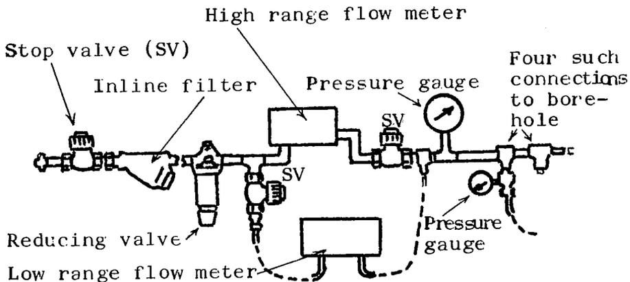
Figure 12. General hydraulic circuitry used at Wentworth instrumented borehole
