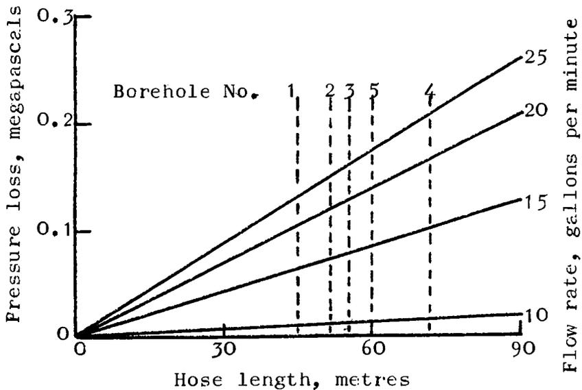
Figure 5. Correction for pressure loss in connecting hosing (Deep Soft test station)
