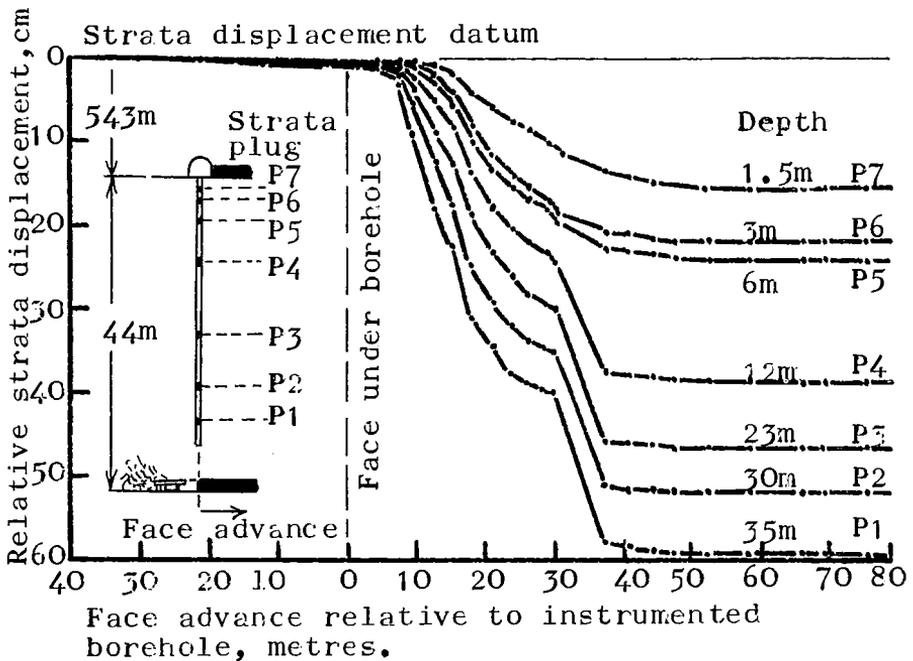
Figure 2. Development of inter-strata displacements in an instrumented borehole located in the path of an approaching longwall extraction. (The illustration has been taken from King, Whittaker and Batchelor (1972)).
