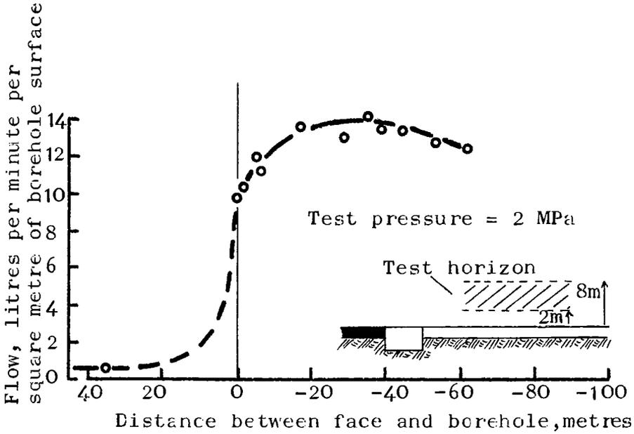
Figure 8. Relationship between flow characteristics of borehole No. 1 and face position
