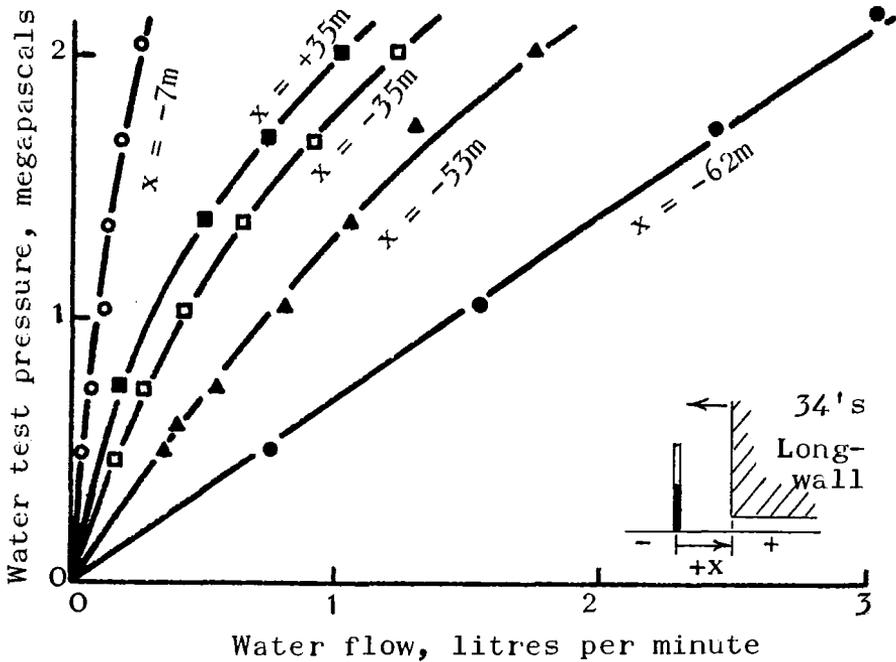
Figure 7. Borehole No.5 flow characteristics.
