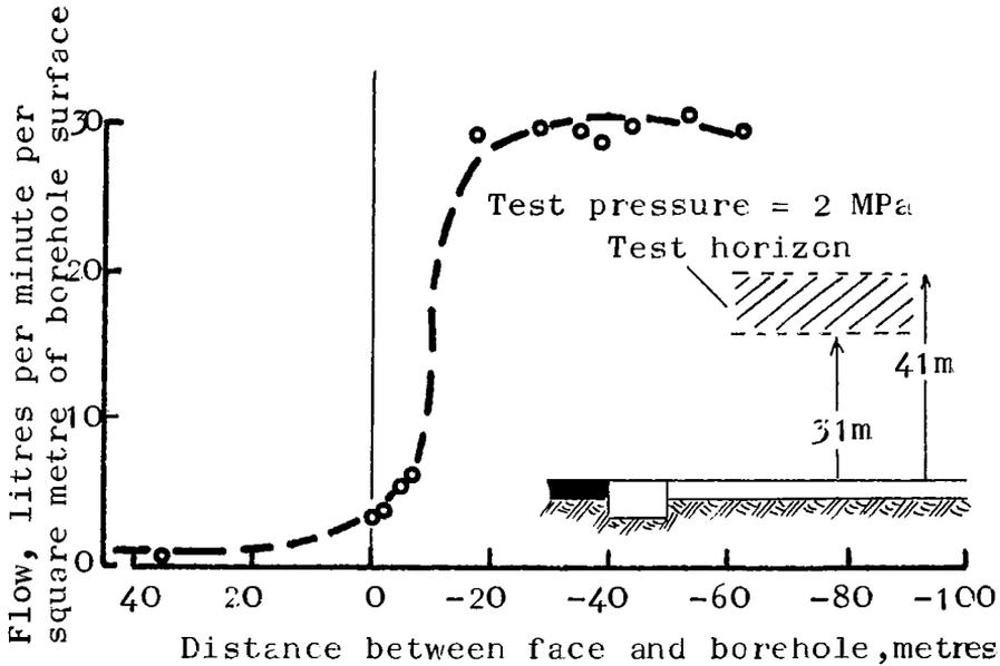
Figure 9. Relationship between flow characteristics of borehole No. 4 and face position
