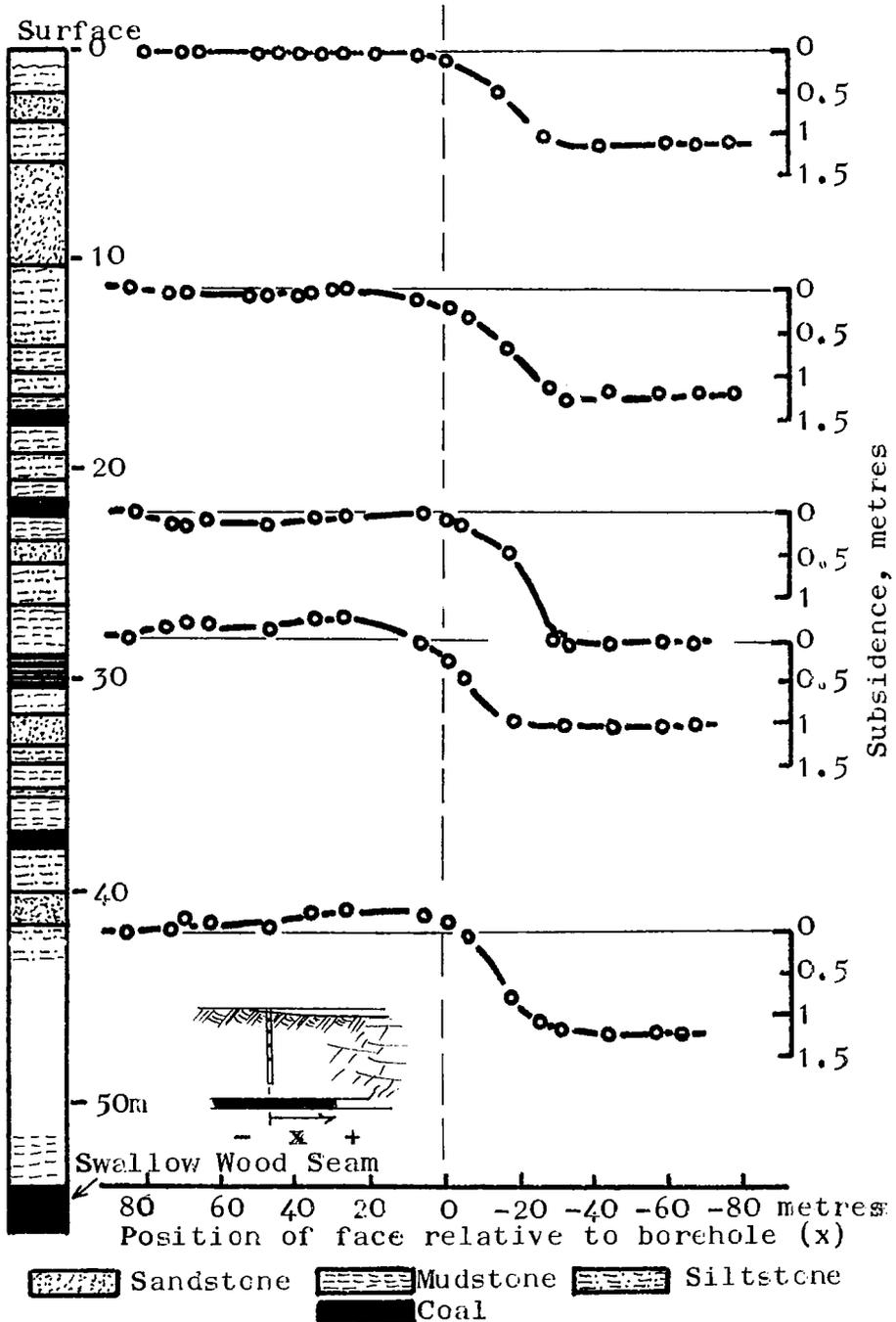
Figure 13. Surface subsidence and sub-surface subsidence characteristics, Wentworth borehole
