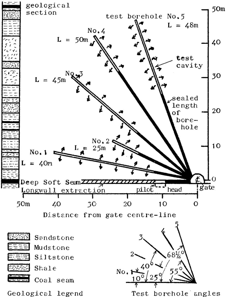
Figure 3. Illustrating positions of test boreholes at experimental site in Deep Soft Seam, East Midlands Coalfield and their location in relation to the Longwall extraction.
