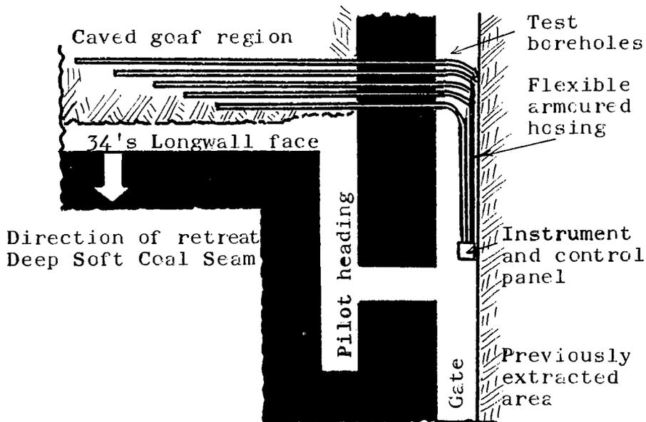
Figure 4. Showing location of test boreholes and instrumentation/test panel
