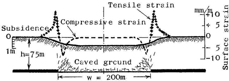
Figure 1. General characteristics of subsidence trough and surface ground strain due to longwall mining of coal seam in shallow conditions. (The subsidence parameters have been calculated using the National Coal Board Subsidence Engineer's Handbook method).
