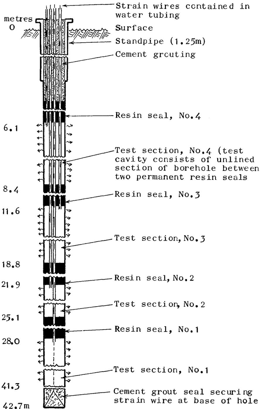
Figure 11. Wentworth instrumented borehole
