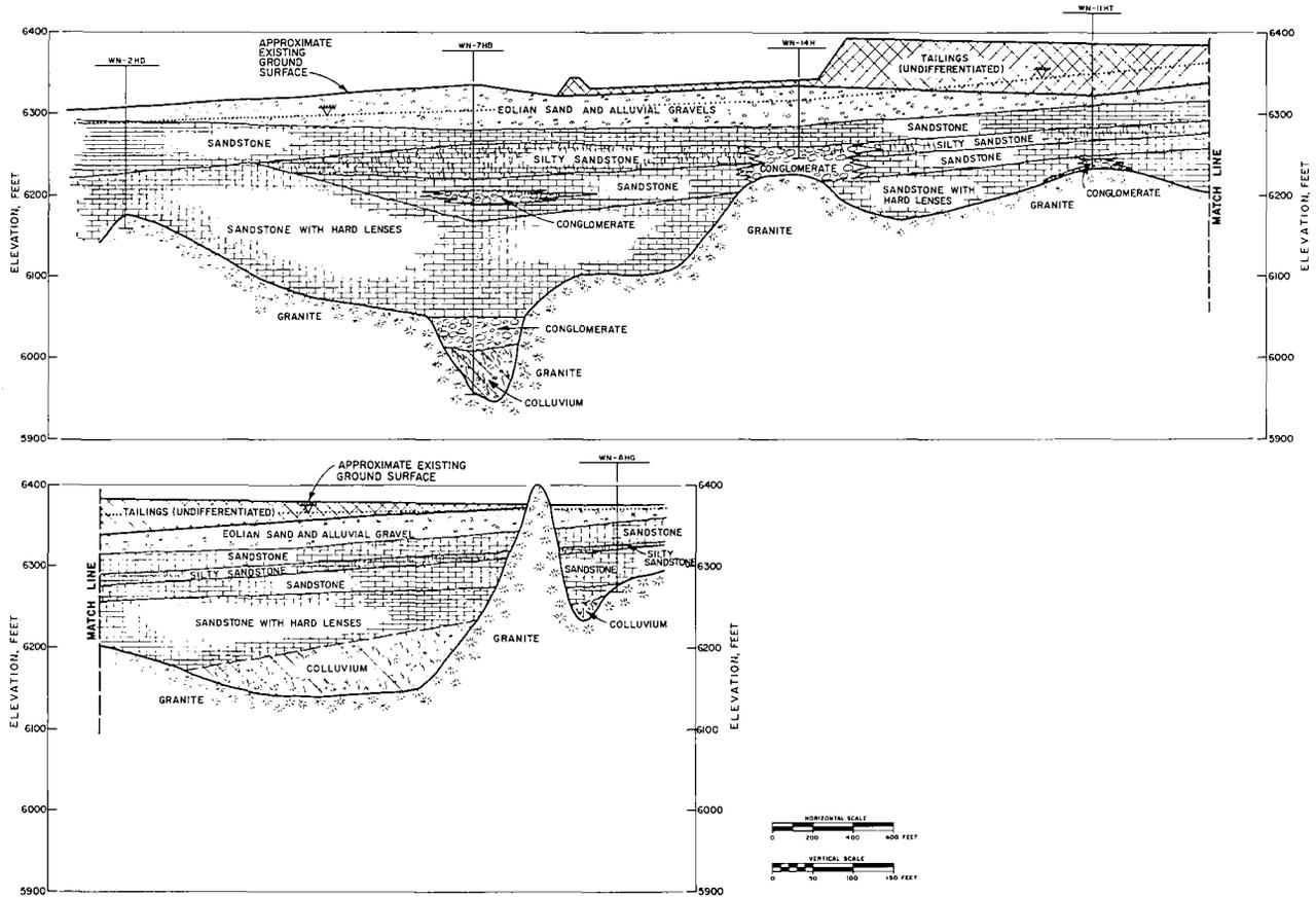
FIGURE 5 SUBSURFACE CROSS-SECTION A-A
