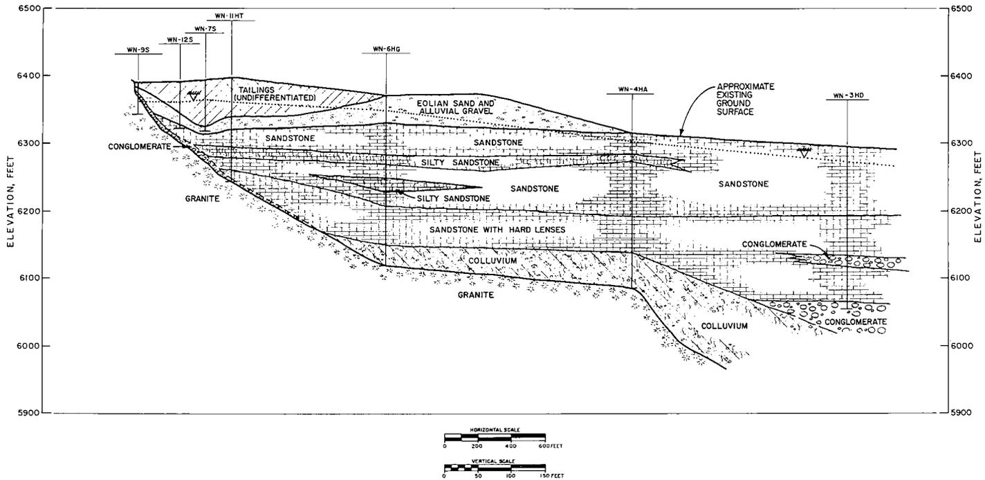
FIGURE 6 SUBSURFACE CROSS-SECTION B-B
