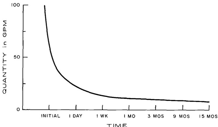
Figure 5. Horizontal Drain Flow Rate.
