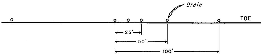
Figure 3. Horizontal Drain Spacing.
