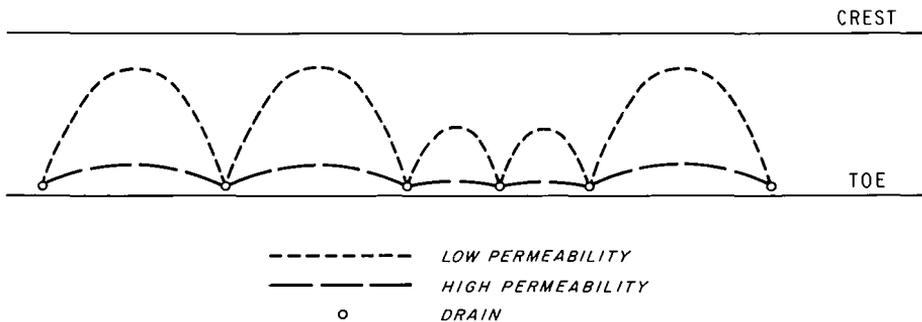
Figure 2. Draw-down Curves Between Drains.
