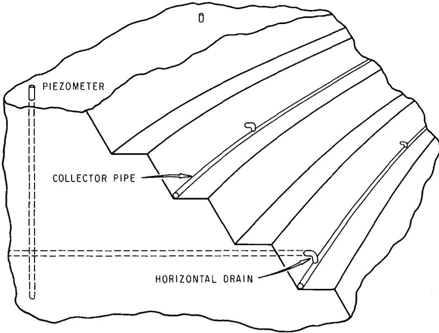
Figure 4. A Complete Horizontal Drainage System.
