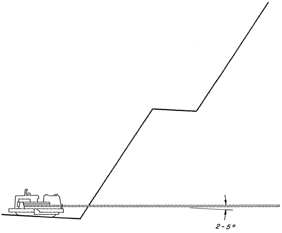
Figure 1. Horizontal Drain Emplacement.
