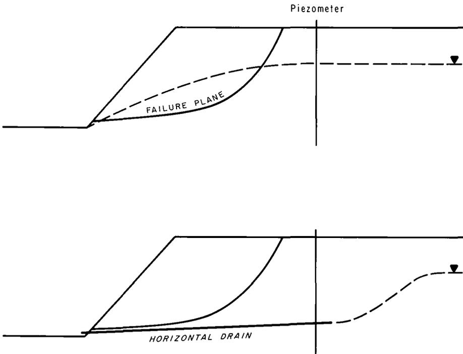
Figure 6. Groundwater Table Location Before and After Horizontal Drain Emplacement.
