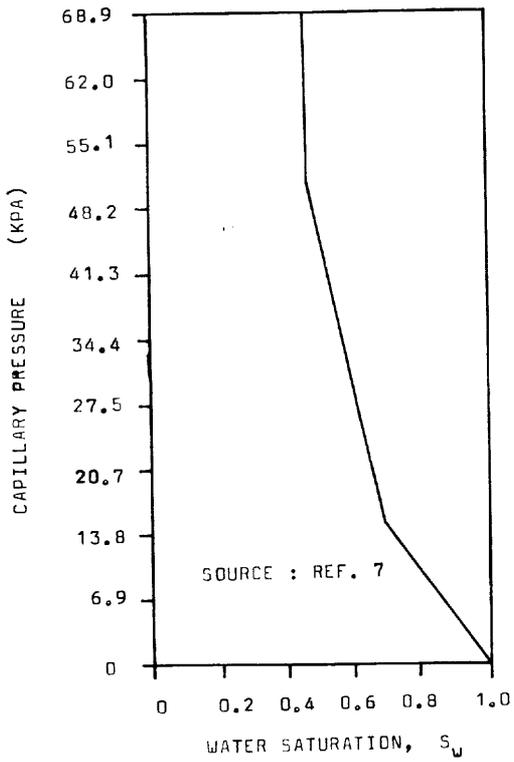
**Figure 2** Capillary-pressure curve used in computer model.
