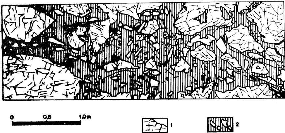
Figure 10. Example of a zone of breccia cemented with calcite. 1. Dolomites, 2. Calcite with fragments of dolomites.
