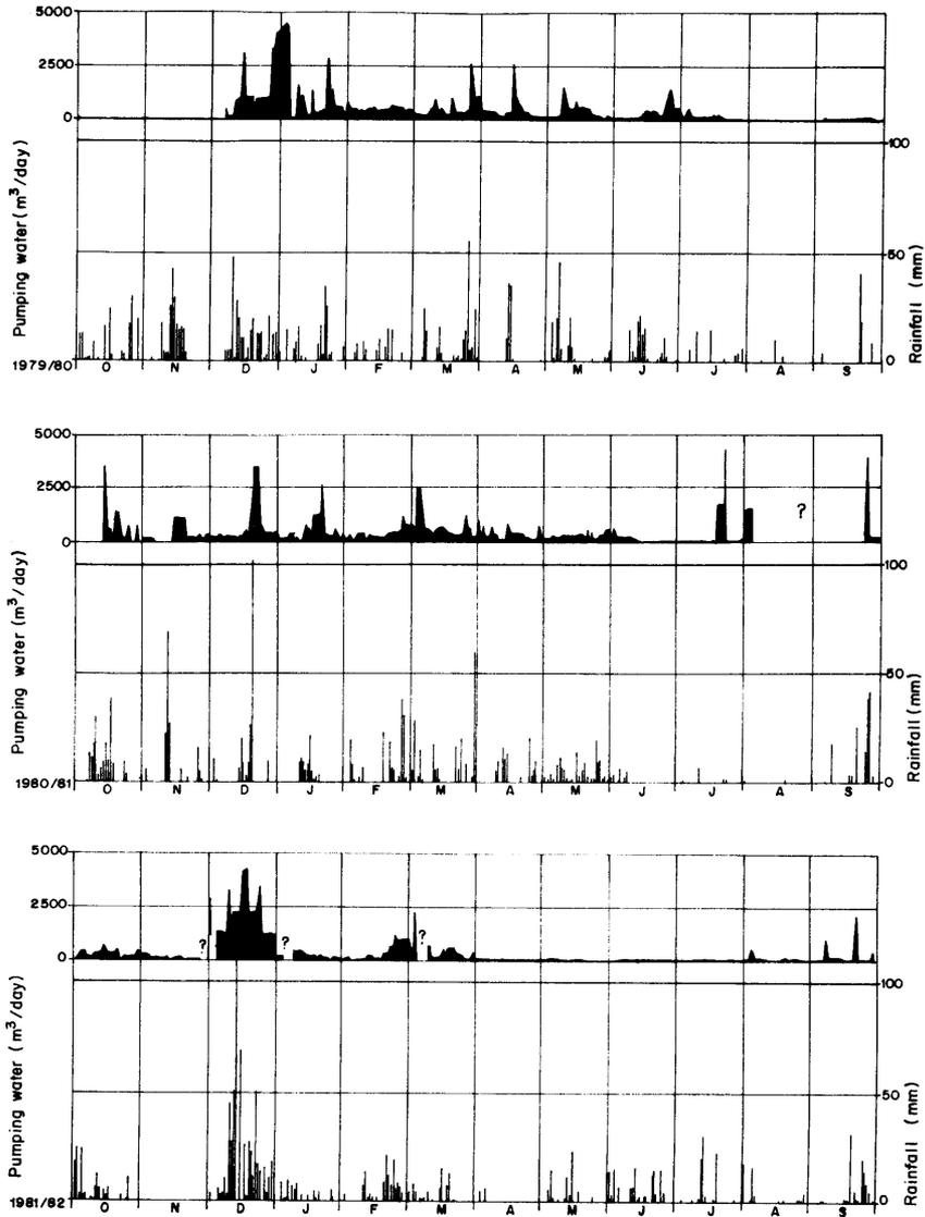
Figure 6. Evolution of pumping water from surface drain against rainfall.
