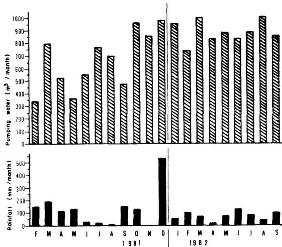
Figure 8. Relationship between monthly rainfall and pumping water from the drainage well.
