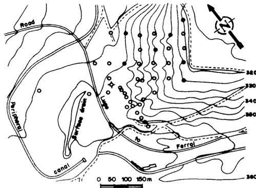
Figure 4. Experimental site for dewatering techniques, with location of peripheral canal, surface drain, pumping well and observation piezometers.
