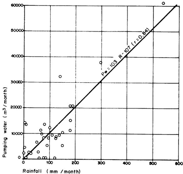
Figure 7. Relation between monthly rainfall and pumping water from the drainage well.
