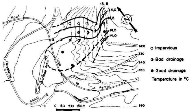
Figure 10. Drainage capabilities in the different piezometers according with the air-lift tests, and isothermic lines of "pumped" water.
