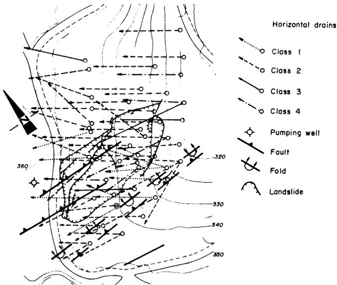
Figure 5. Horizontal drains (boreholes), classified by categories according with their water yield.
