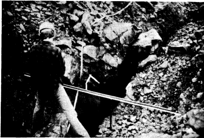
Figure 2. Monitoring movement across tension cracks. The cracks should be filled with impervious material to prevent high water pressure buildup behind the slide.
